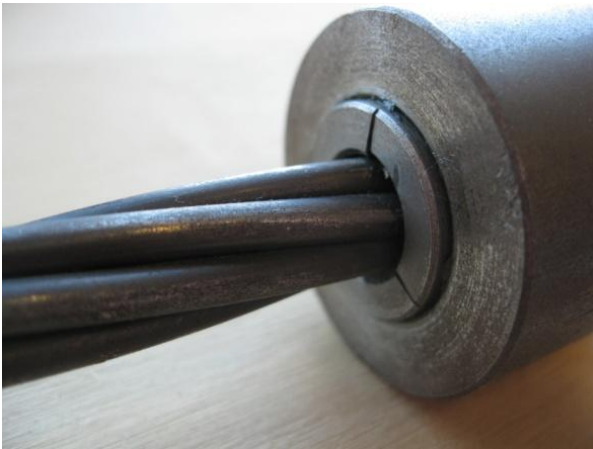
Figure 10: Post-tensioning tendon, and barrel and wedge system used for full scale testing
