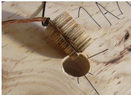
Figure 6: Thermocouple plug and associated hole
