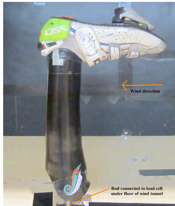
Figure 7.37: Set up of Lower Leg Model in the High Speed Wind Tunnel
