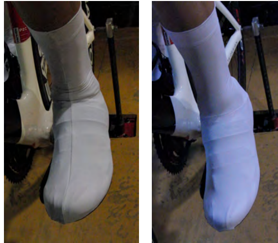
(a) Prototype 1: Seam down the front (b) Prototype 2: Seam across the ankle
