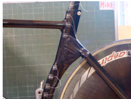
(c) Seat tube modification
