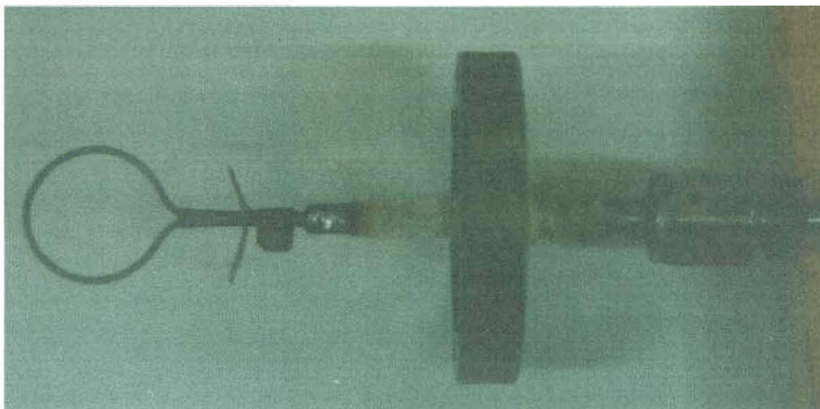
Figure 2.1. Photograph of the ring inlet used for neutral addition to the SIFDT.
