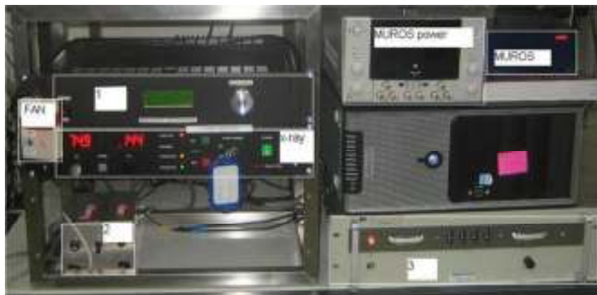
Figure 3.3 The MARS-CT scanner show the main components, (1) Motor controller, (2) Fan switch, (3) Power supply, and as labeled the x-ray control and MUROS readout.
