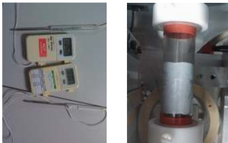
Figure 8.3 The thermocouple placed in the scanner to measure the temperature variation when the scanner at operation.
