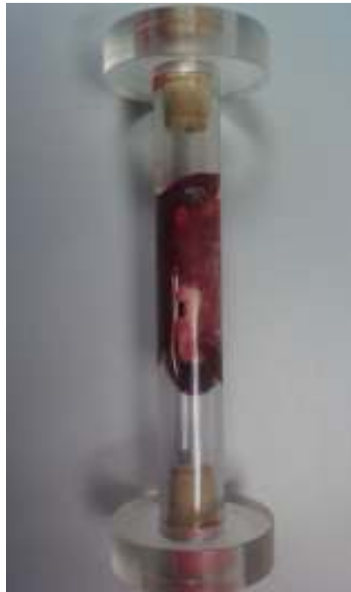
Figure 8.1 The prepared sample, showing the tube holding the fat and liver, which are separated by a paper clip.
