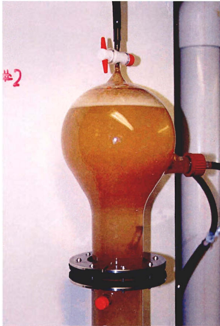
Figure 7-9 FBR2-2(b) with foam at the top of the settling chamber.
