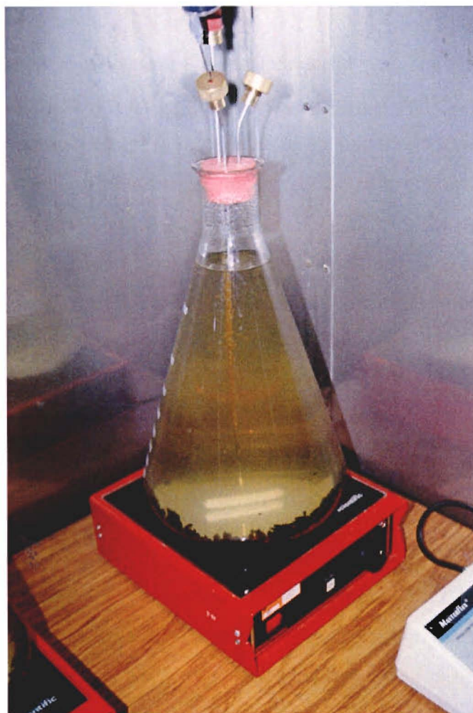
Figure 5-3 Pretreatment Batch Reactor 1f, coconut shells (2-8mm, air dried) in deionised water.
