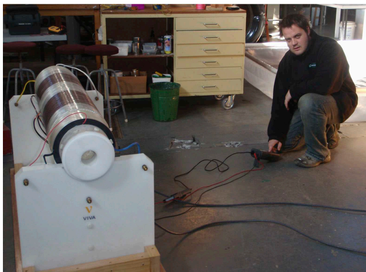
Figure 4.10 Testing the Manapouri Partial-Core Transformer.
