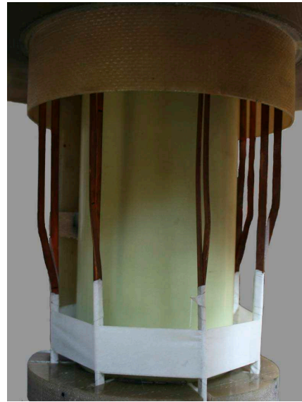
(b) The upper portion of the copper lead-outs.
