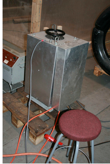
(a) Main measurement and control desk. (b) The variac used to control the supply to the HTSPCT.
