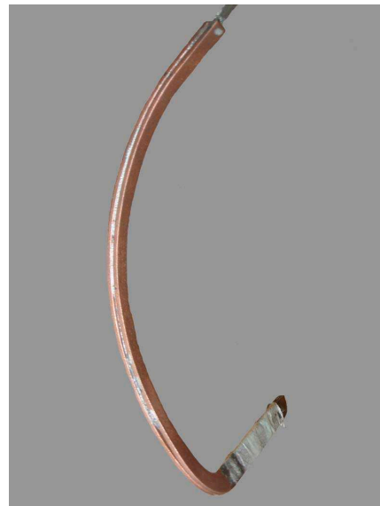
(d) Photograph of a sample joint between the copper lead-outs and the HTS wire.
