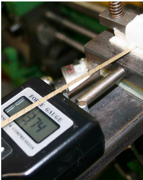
(c) The force gauge used to measure the wire tension.
