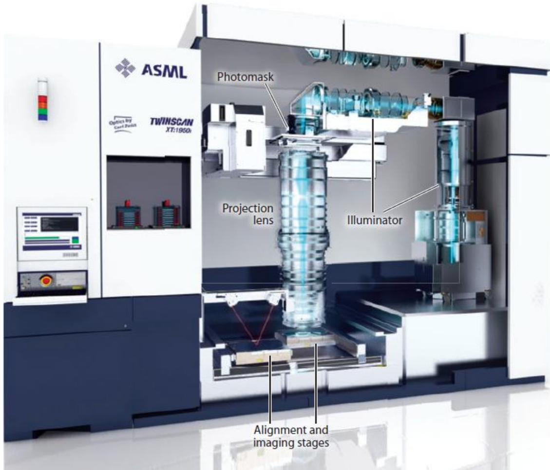
Figure 2-3 – ASML TwinScan XT:1950i – A state of the art water immersion stepper for the sub-32 nm node, designed for a NA of 1.35 operating at the ArF, \lambda = 193 nm. It has a throughput of \sim 140 wafers/hour [30-31]
