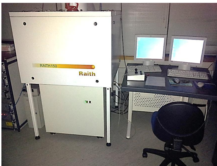
Figure 3-31 – Photograph of the Raith 150 EBL system that doubles as a Scanning Electron Microscope
