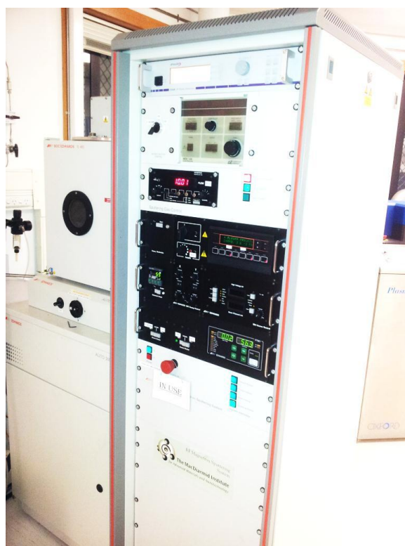
Figure 7-3 – Photograph of the Edwards system. The RF magnetron sputtering module was used to deposit thin films of HfO
