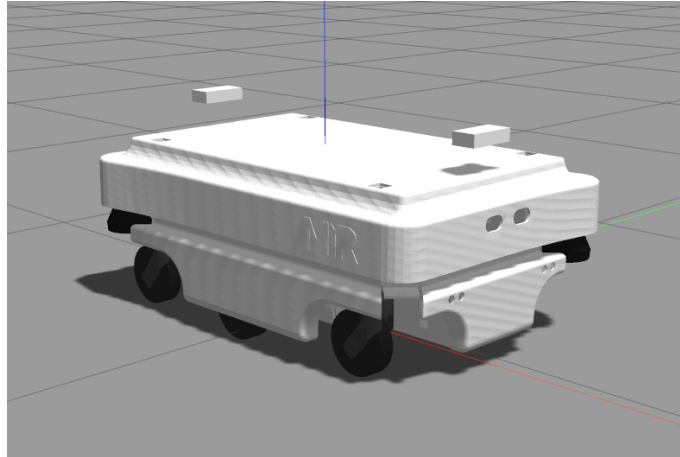
Figure 3.15. The modified MiR robot with cameras.
