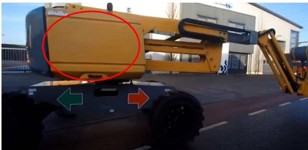
Figure 2. Location of the Engine and the pump in the HA16 RTJ PRO
