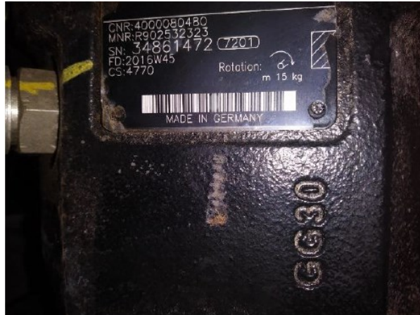
Figure 4. Manufacturer's plate of the main pump. Figure from [2]
