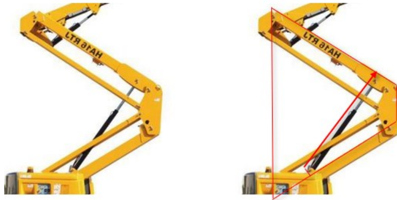
Figure 27. Lower boom structure and its simplification draw (in red)
