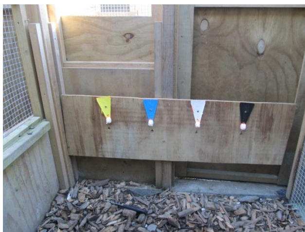
Figure 2.1: Colour preference testing was conducted by painting the plastic backing of Waxtags® and evenly spacing them along a wooden board.
