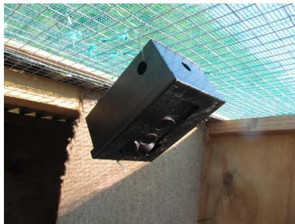
Figure 2.8: The Acorn LA series camera (Viewtech Ltd) inside a metal security case (to prevent animal damage) positioned on the possum enclosure wire roof to capture animal’s interactions and behaviour towards devices.
