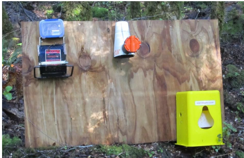
Figure 1.1: Three possum traps commonly used in New Zealand, from left to right the Warrior, Henry and Timms traps.
