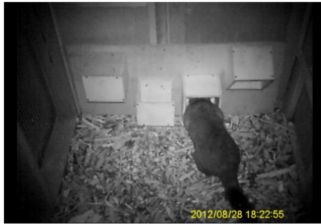
Figure 2.7: Cameras were positioned at a high angle to record possum approach behaviour while also giving a clear field of vision of interactions with each device. Above is an example picture capturing a possum removing bait from the ‘Timms’ design during landscape position testing on the night of the 28 th August, 2012.
