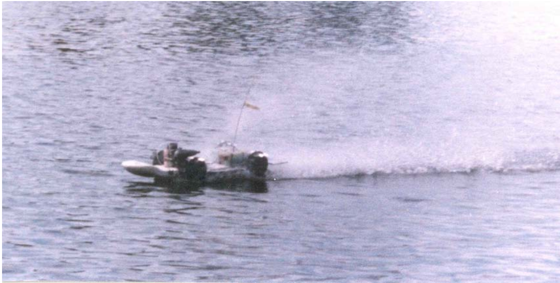
Figure D-1. Radio controlled LPW model in the planing-flying condition at about 9m/s (32kph) 1 .
