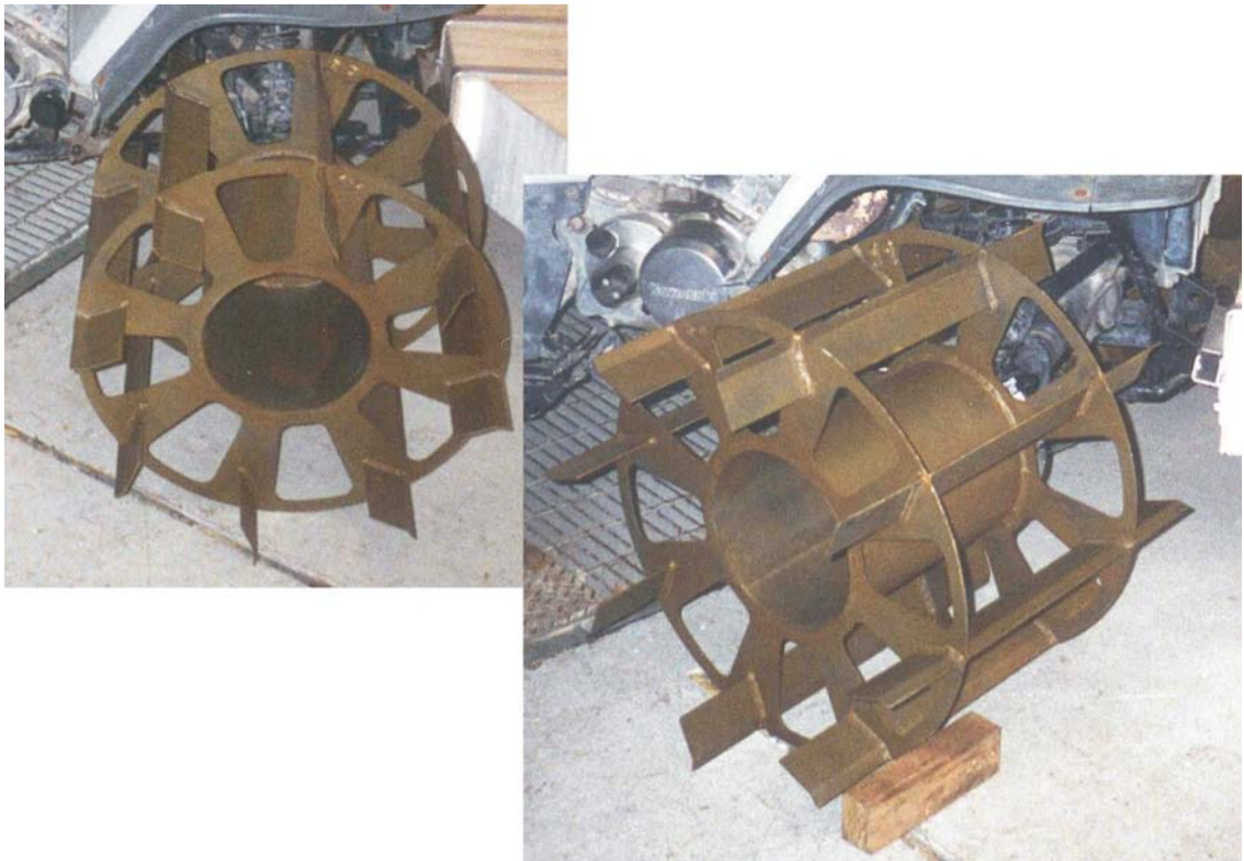
Figure 1-1. Right front LPW as used on KLF400 prototype. Forward rotation to the right.
