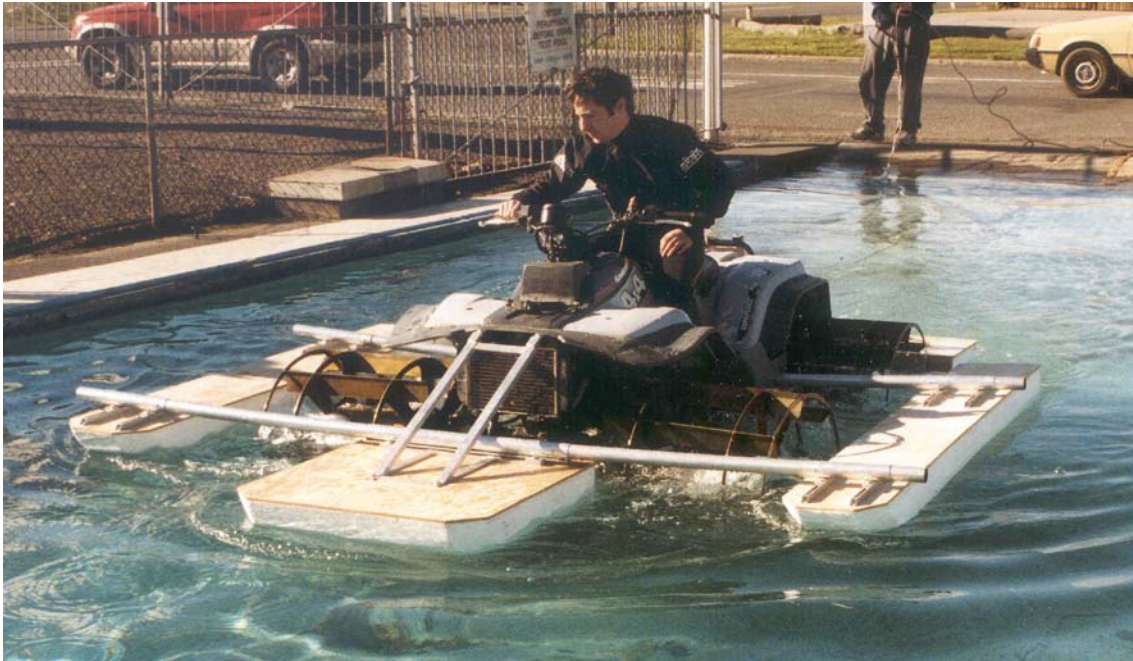
Figure 5-1. Pool test. Note the immersion ( d/D ) is greater than 0.5. Lack of strut bracing allowed flexing of the side float mounts, increasing immersion depth.
