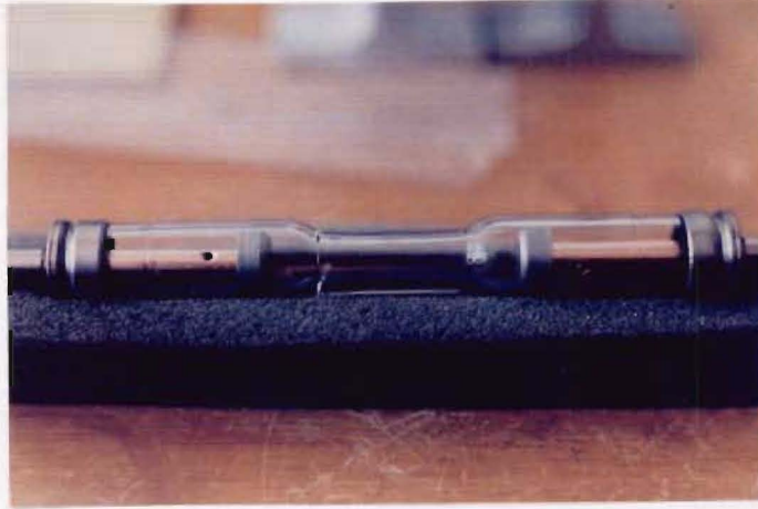
Figure 8.3: The xenon flash-tube used for the first part of the trial. (0.7x actual size)
