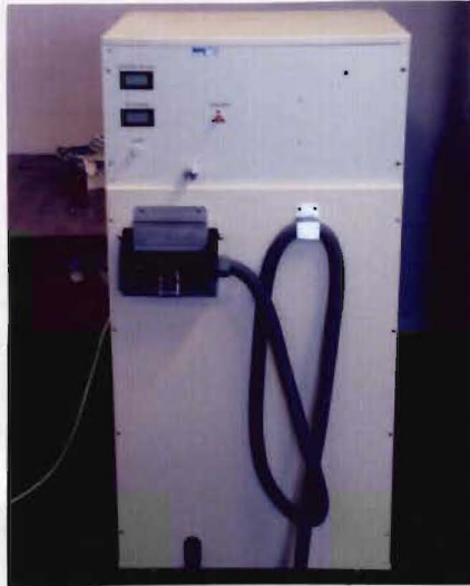
Figure 8.15: The second prototype of the flash-lamp tattoo treatment system.
