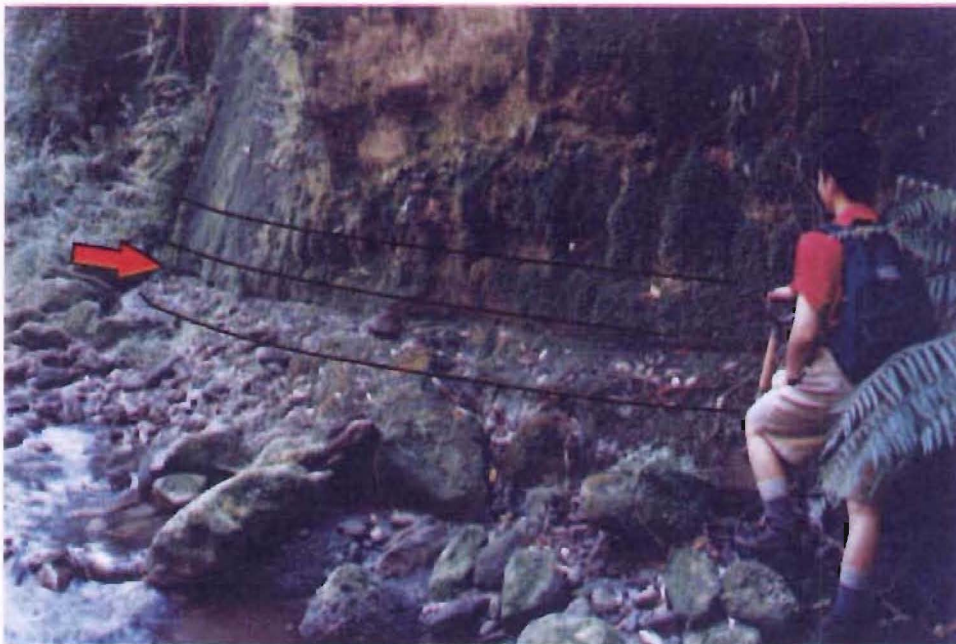
Figure 4.24 Flexural shear defect sub-parallel to bedding
