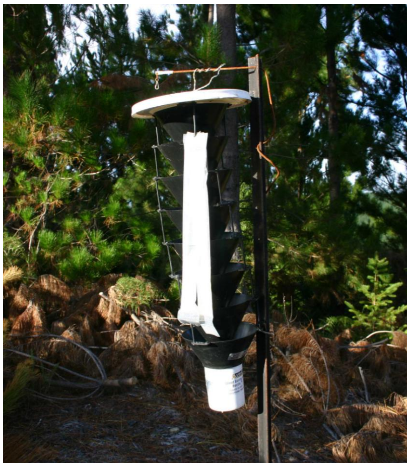
Figure 2.3. Lindgren-type funnel trap, with dispensers for attractant ( \alpha -pinene and ethanol) on the side (see text).
