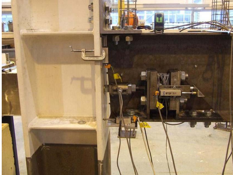
Figure 2: Steel Joint with HF2V Device Setup
