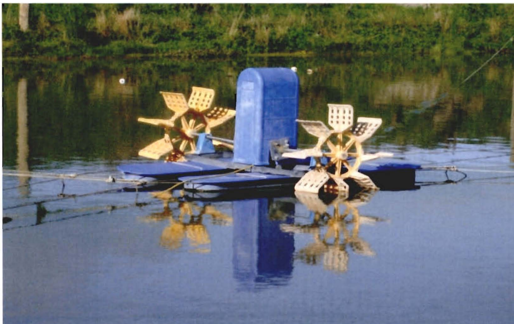
Figure 12: Picture of the mechanical paddlewheel aerator used to maintain high dissolved oxygen levels.
