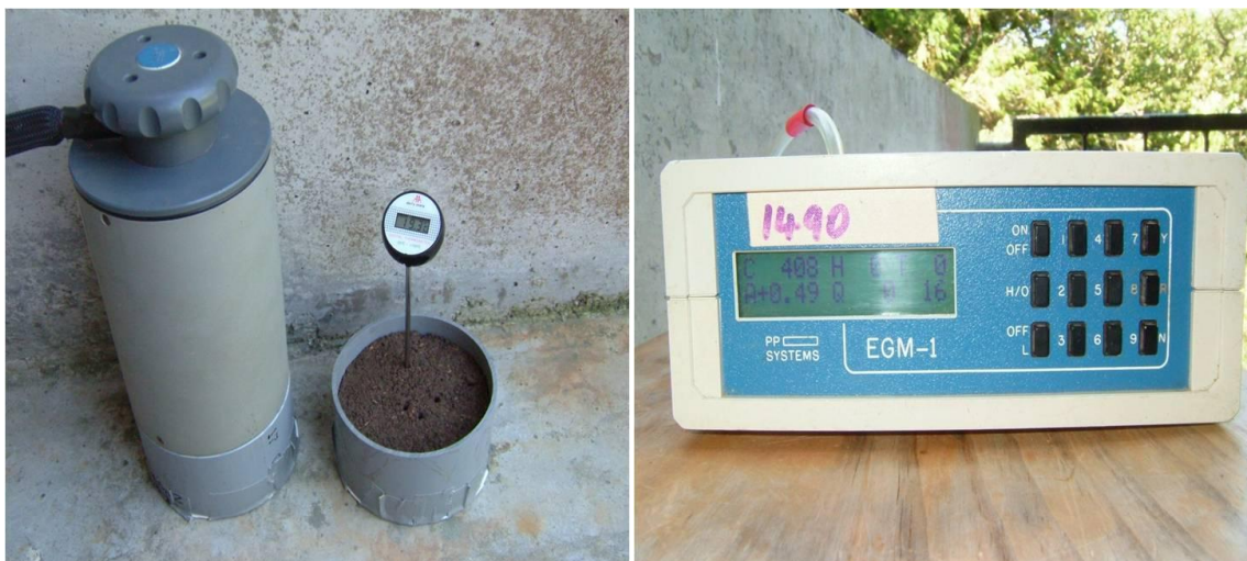
Figure 6.2 Portable chamber with an infrared gas analyser.
