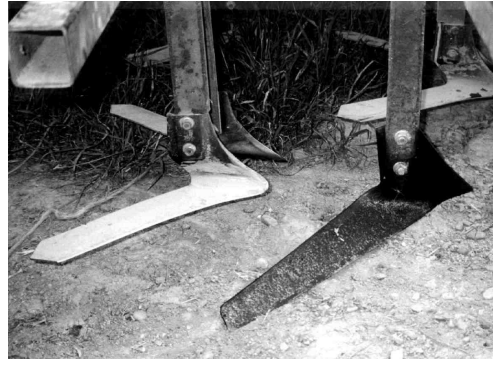
Figure 4. Poorly designed hoe blades
