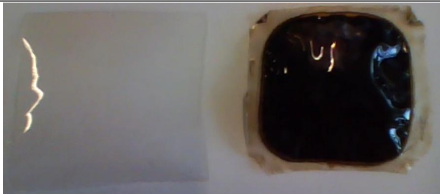
Figure 3.7: Fouling of proton exchange membrane. An unused PEM (left) is compared to a PEM (right) that has been used in a MFC for a combined total of 40 h of experimental time.
