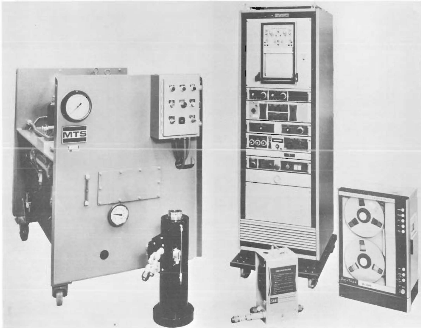
FIGURE 2-1 : MTS MODEL 903.79 STRUCTURES TESTING SYSTEM
