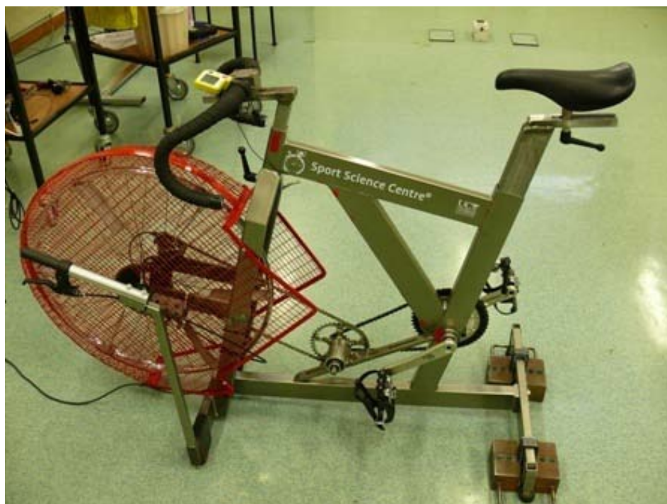
Figure 7. Repco Cycle Ergometer used for the 30s-WAnT for determination of anaerobic capacity.
