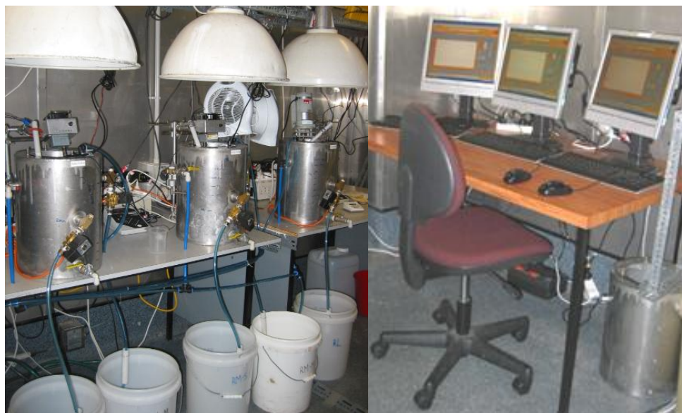
Figure 5-1. Tri-SBR Setup (Left) and Data Logging and Control Interface (Right) for Retention Time Experiments within Controlled Climate Laboratory Room.
