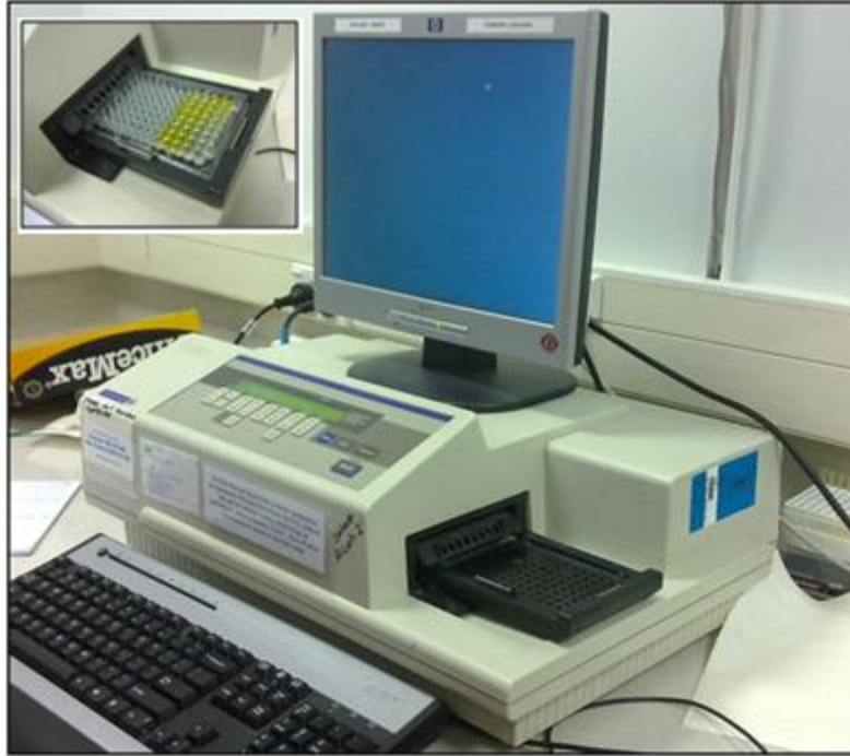
Figure 2.6: Microplate reader for ELISA development kit to measure natural and recombinant human Vascular Endothelial Growth Factor (VEGF). Insert: 96-well microtitre plate before development.
