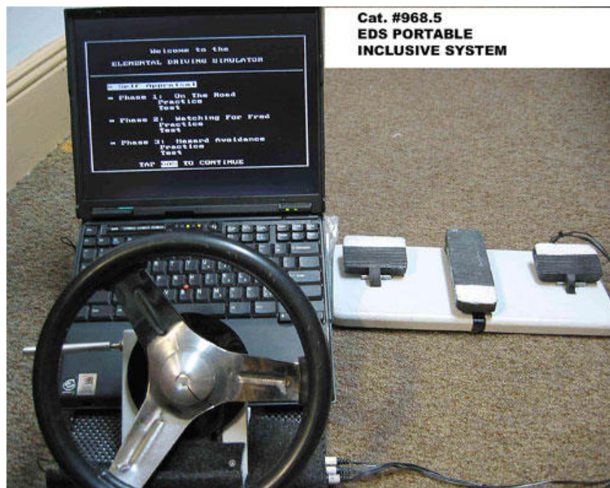
Figure 3-3. The EDS Portable Inclusive System showing computer, steering wheel with indicator stalk to the left, and foot pedals.
