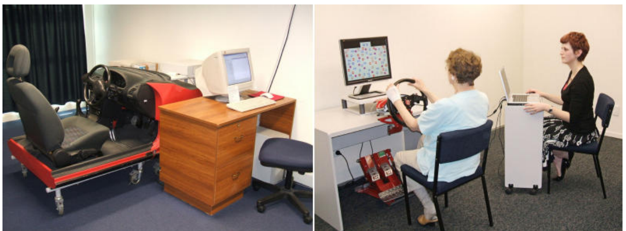
Figure 3-4. The modified car body used to run SMCTests pictured left. Test stimuli are projected onto the white wall in front of the machine. The semi-portable CanDAT apparatus is pictured right.
