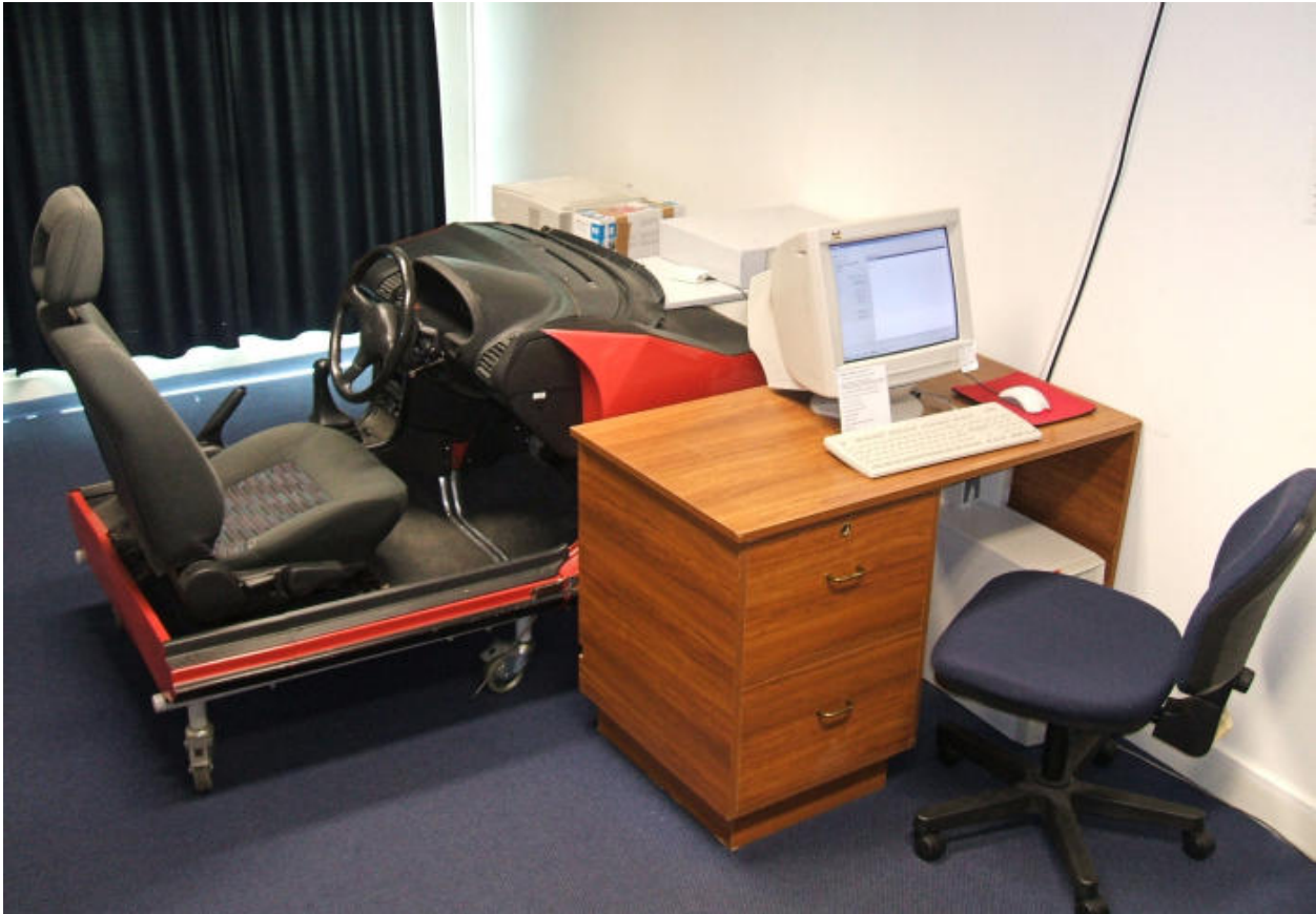
Figure 5-3. The modified car body hardware running SMCTests software used for The Dementia and Driving study. During testing room lights are switched off and test stimuli are projected onto the wall in front of the apparatus.
