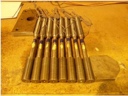
Figure 6.4 a) mild steel energy dissipater; b) completed joint assembly with bracket and dissipater
