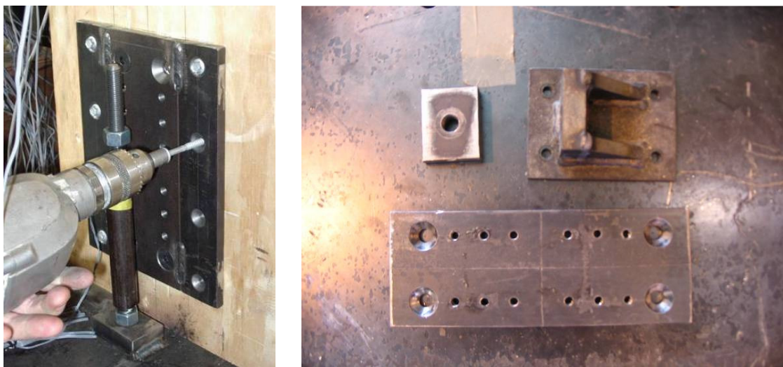
Figure 4.9 Attachment details of energy dissipaters to walls
