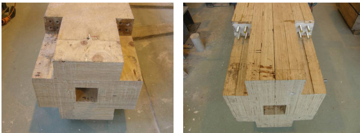
Figure 6.2 Beam end before and after insertion of epoxyed threaded bars
