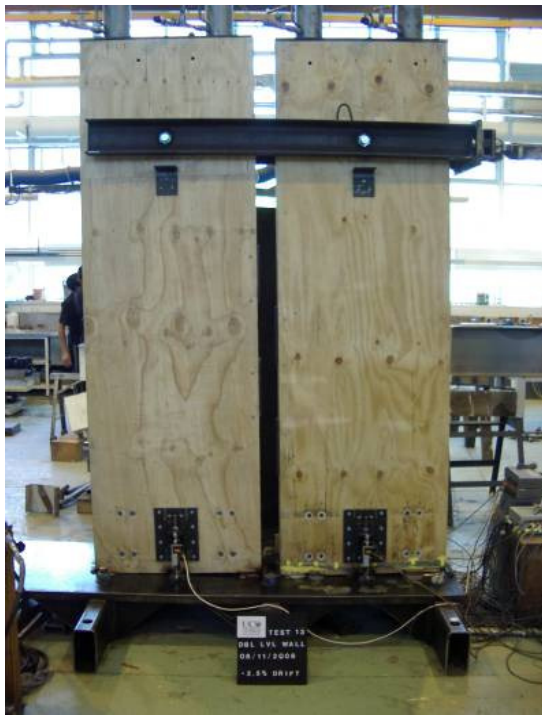
Figure 8.4 View of walls with axial dissipaters a) test specimen b) with dimensions
