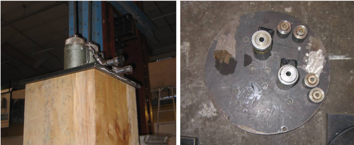
Figure 5.4 View of loading jacks and anchorage at top
