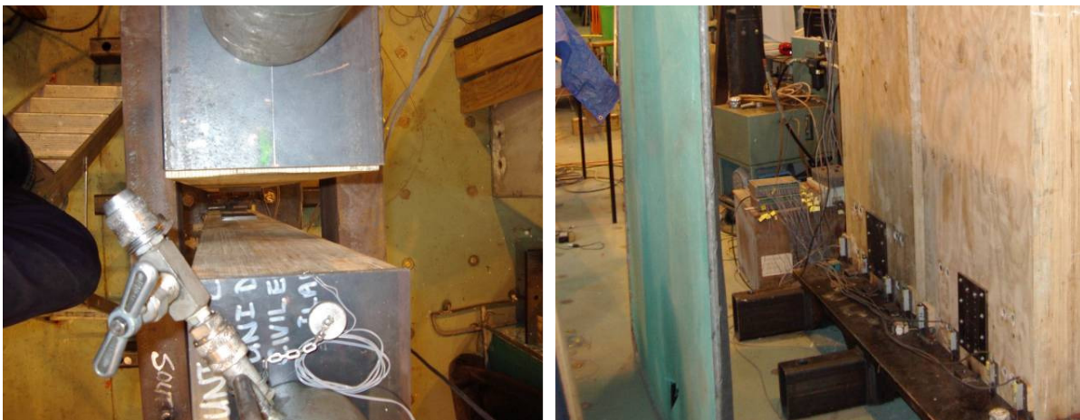
Figure 4.8 Gap between the wall as seen from the top and rear view of the walls with instrumentation
