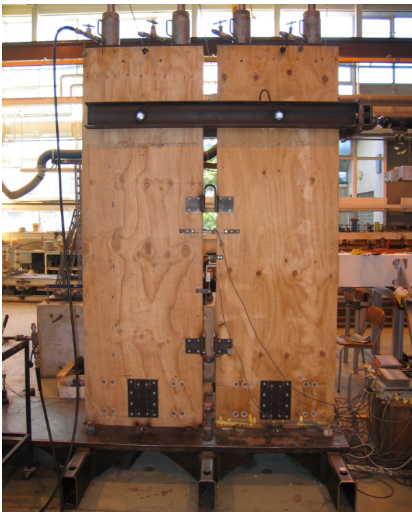
Figure 4.15 Hybrid LVL walls with UFP
