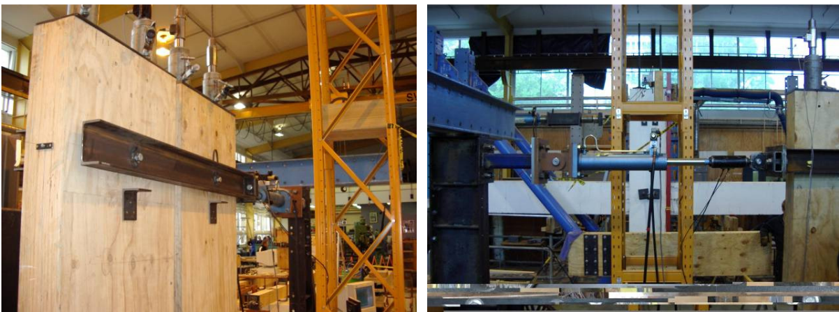
Figure 4.7 Steel loading beam with pin connections and loading jack
