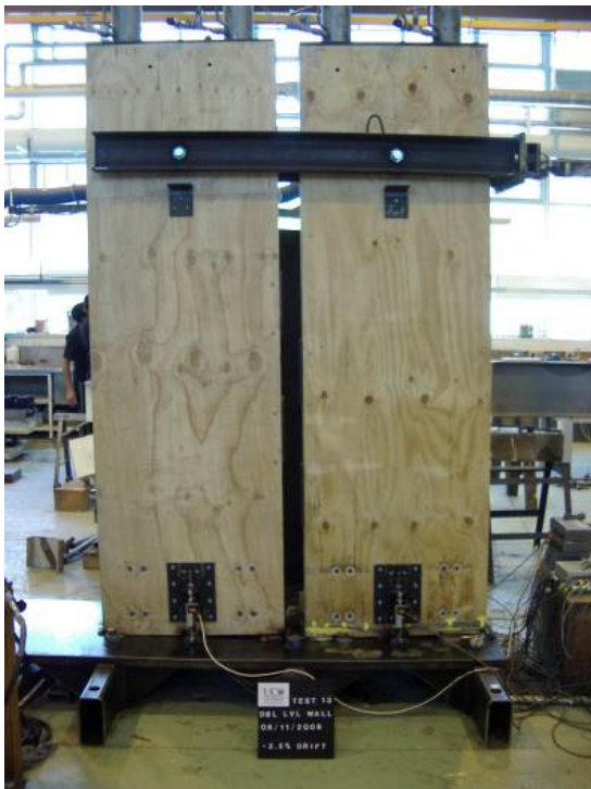
Figure 8.25 View of walls with axial dissipaters a) test specimen b) with dimensions
