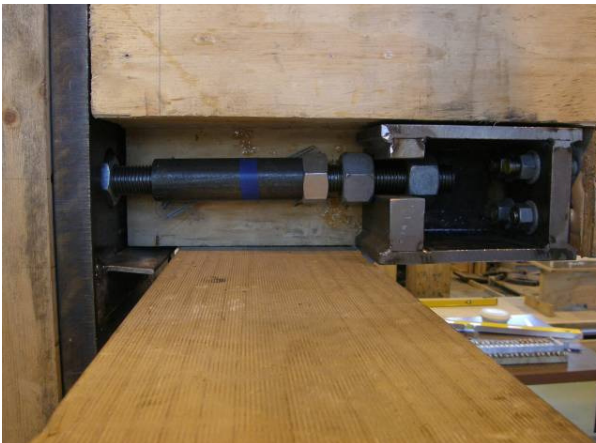
Figure 6.5 Close-up views of dissipater connection through bracket, nuts and washer
