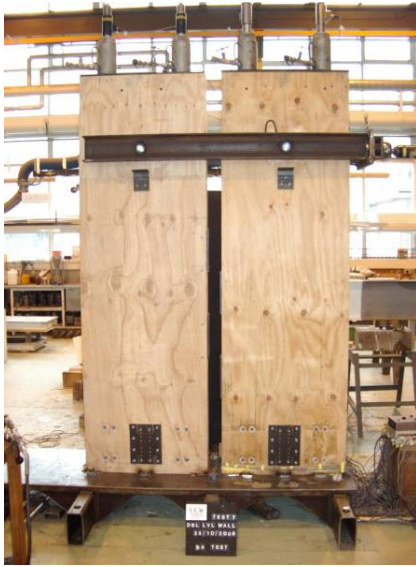
Figure 8.24 View of PT-only walls a) test specimen b) with dimensions
