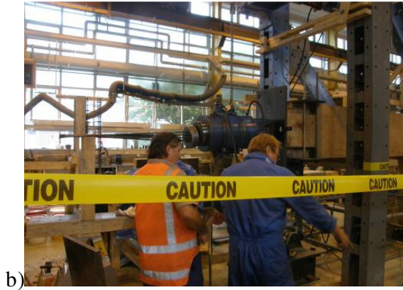
Figure 6.3 a) components of beam-column joint assembly; b) post-tensioning of test specimen
