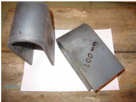
Figure 4.11 U-shaped flexural plates with attachments
