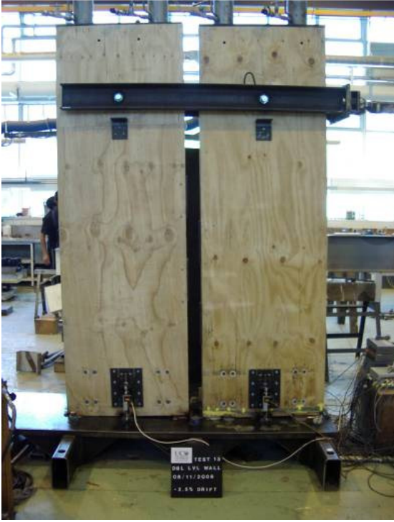
Figure 8.3 View of walls with axial dissipaters a) test specimen b) with dimensions
