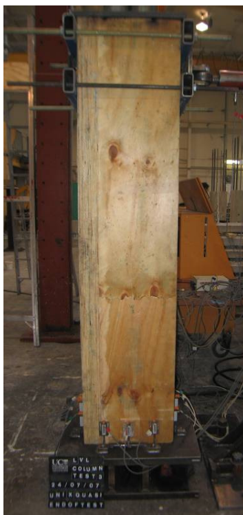
Figure 8.9 View of PT-only column a) test specimen b) with dimensions
