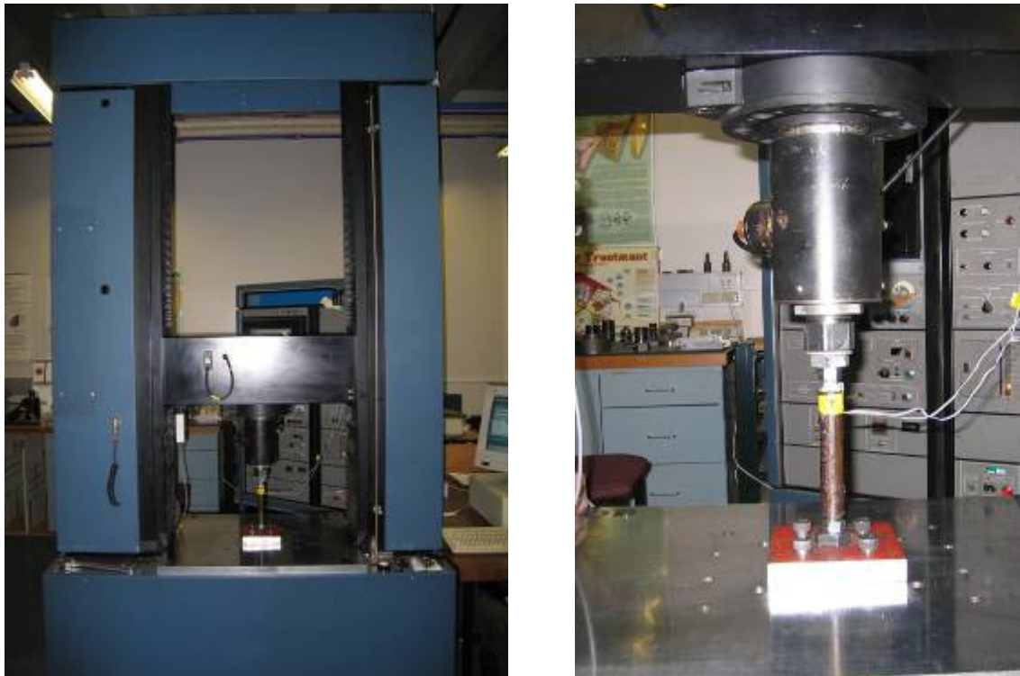
Figure 4.16 Test setup for axial dissipaters
