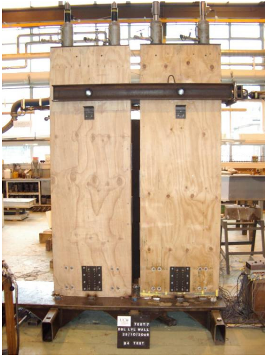
Figure 8.1 View of PT-only walls a) test specimen b) with dimensions
