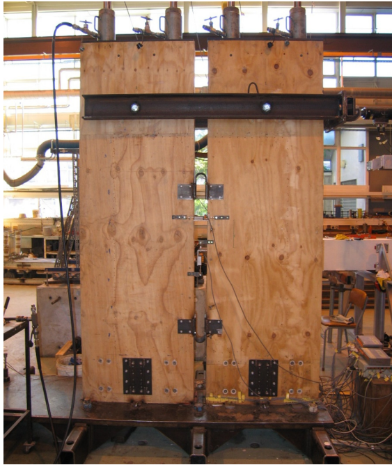
Figure 8.7 View of walls with UFP dissipaters a) test specimen b) with dimensions
