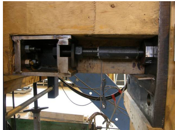
Figure 6.5 Close-up views of dissipater connection through bracket, nuts and washer
