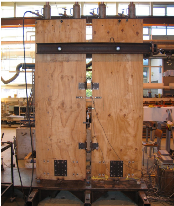
Figure 8.26 View of walls with UFP dissipaters a) test specimen b) with dimensions
