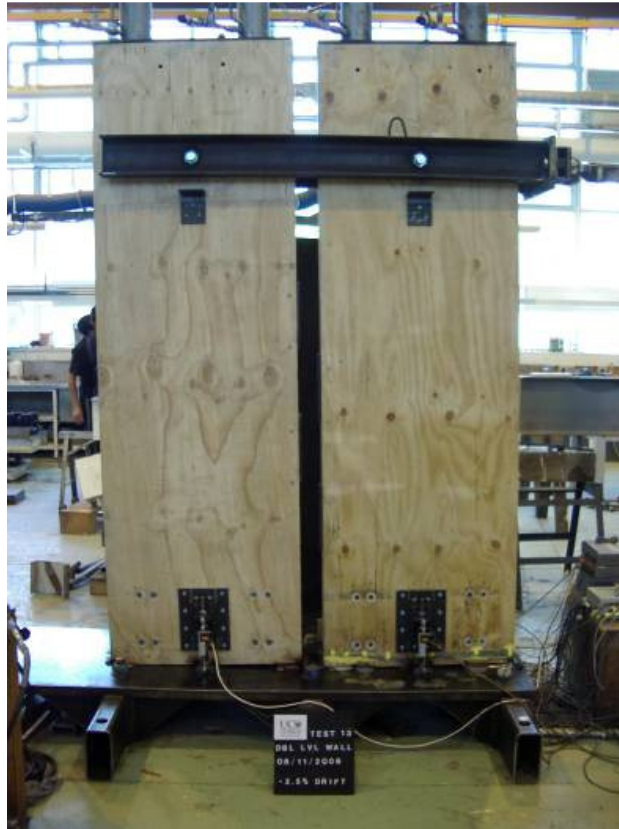
Figure 4.10 Hybrid LVL walls with axial dissipaters
