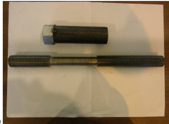
Figure 6.4 a) mild steel energy dissipater; b) completed joint assembly with bracket and dissipater
