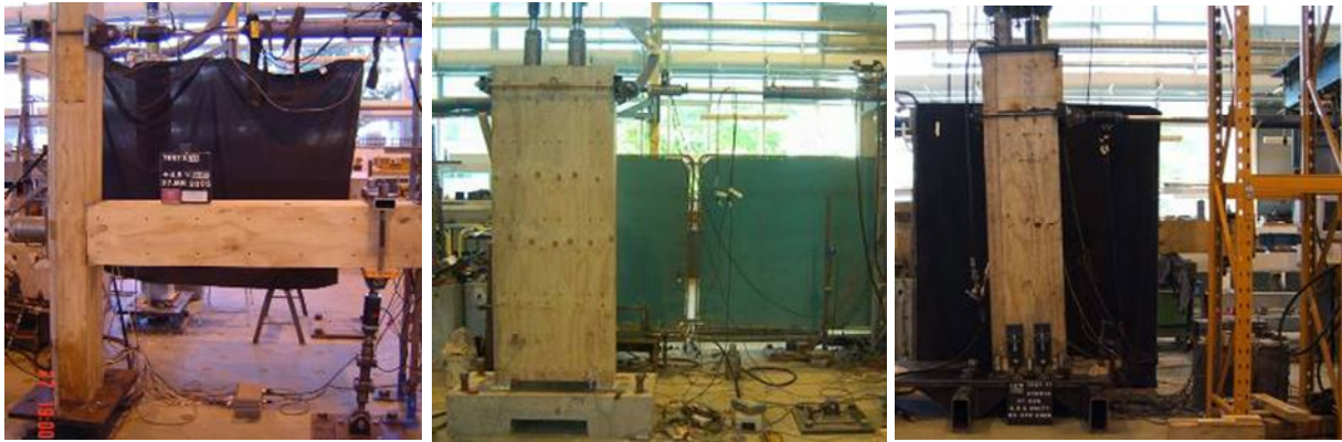
Figure 2.19 Beam-column joint, wall and column test specimens (Palermo, et al., 2006c)
