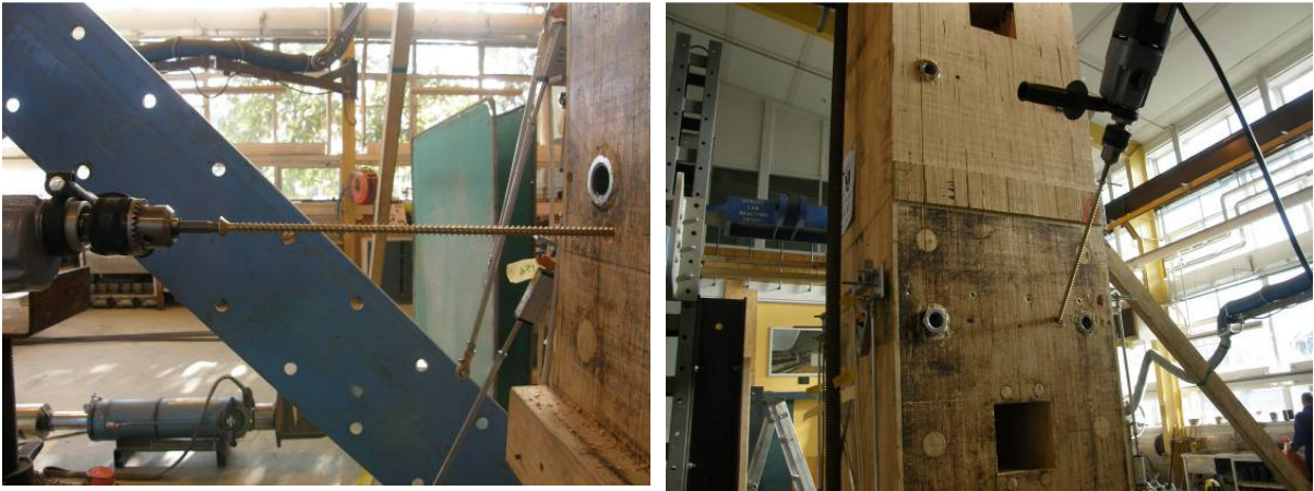
Figure 6.20 Horizontal and Diagonal screws inserted into the column
