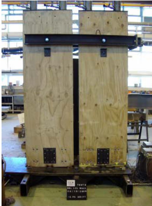
Figure 4.4 View of LVL walls
