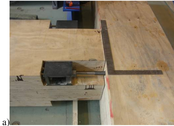
Figure 6.3 a) components of beam-column joint assembly; b) post-tensioning of test specimen
