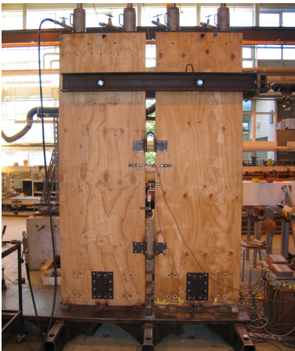
Figure 8.6 View of walls with UFP dissipaters a) test specimen b) with dimensions
