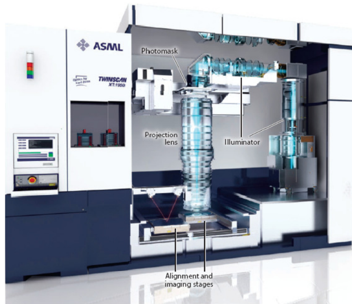
Figure 1.4 ASML Twinscan XT:1950i scanner, a modern day lithography machine capable of imaging >140 wafers per hour. The illuminator (source), lenses, photomask and stage (substrate) are labeled [French 2009]
