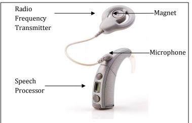
Figure 5: External components of a cochlear implant (New Zealand Audiological Society, 2010)
