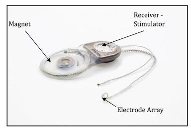
Figure 6: Internal package of a cochlear implant (New Zealand Audiological Society, 2010)
