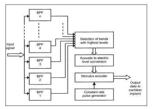
Figure 8: Diagram of the Advanced Combination Encoder (ACE) speech processing strategy (McDermott, 2004)
