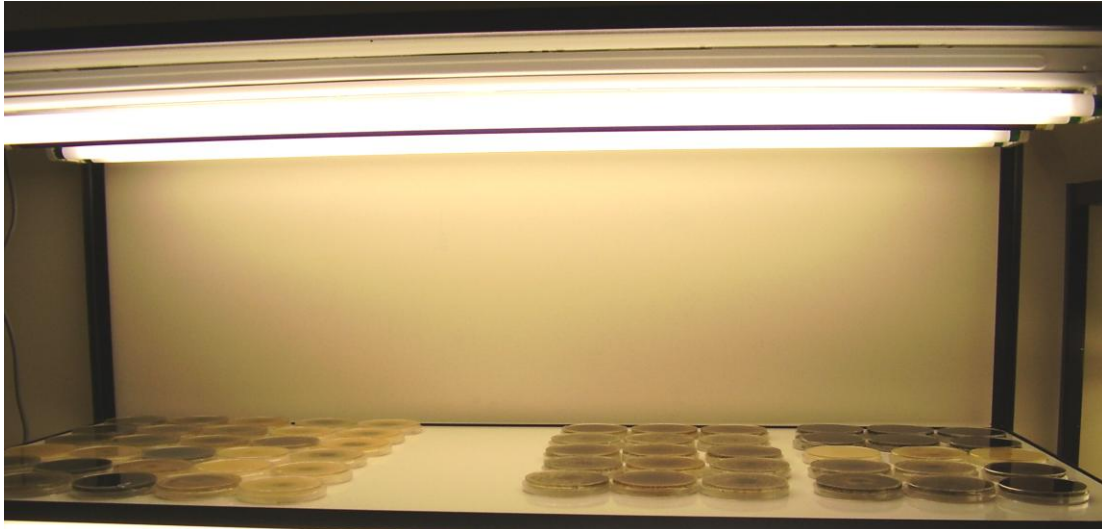
Figure 2.3: Layout of fluorescent light beams used to produce near UV light to induce the in vitro sporulation of botryosphaeriaceous species. Lights are 75 cm from the surface of the plates. The light overhead beam consisted of four 40 W cool white fluorescent bulbs (Philips TLD 36W/840) arranged by two on each sides with a single 36 W blue bulb (SYLVANIA FL36W/ Blacklight blue) in the centre.
