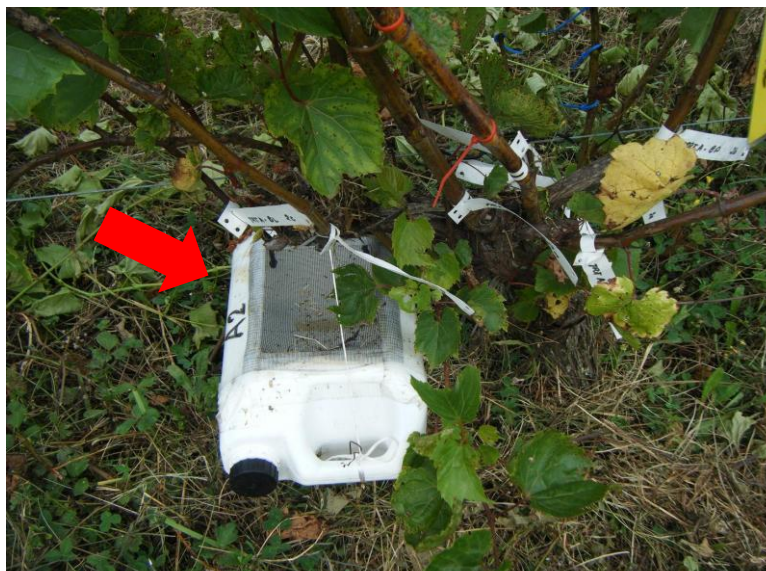
Figure 5.2 Rainwater run-off traps made of 5 L plastic container (arrow) installed underneath the canopy of a rootstock mothervine.
