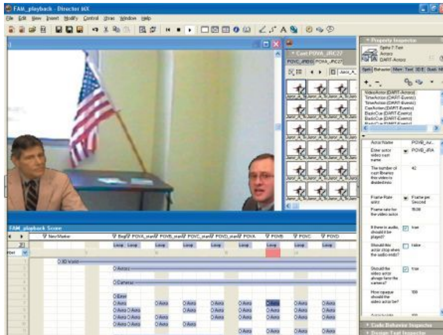
Figure 2.4: An Example Work Session in DART (while debugging the Four Angry Men (FAM) experience). The entire score for FAM is visible, including the nine scenes and most of the actors. The stage (containing the running experience) is visible, as is part of the content for one video actor, and some of Director’s editing windows. (Image from MacIntyre et al.)
