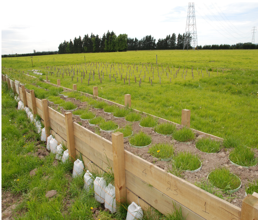
Plate 5.2. Lysimeters installed in field
