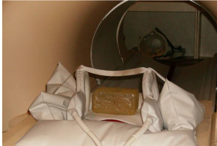
Figure 5- 52 Another view of the same experimental set up for the vertical bristle gelatin phantom while it has been flipped 90^\circ to obtain multiple measurements in 3-D from this orthotropic composite-like sample.
