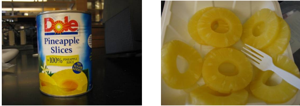
Figure 5- 38 A circular slice of pineapple provided from a cane was used to fabricate the pineapple gelatine phantom for the orthotropic MRE testing. Different fibre orientation with different length in the pineapple can be observed.
