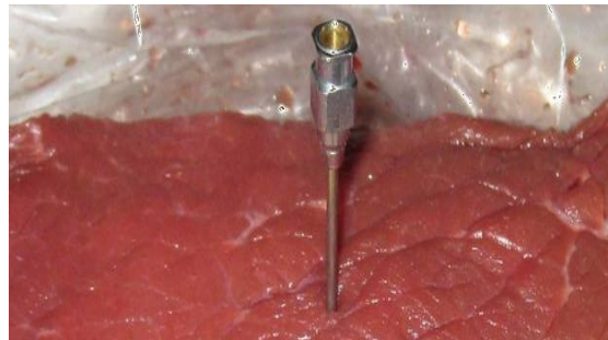
Figure 5- 9 The metal needle shown in this picture was used to facilitate locating the single-mode fiber through the muscle phantom.
