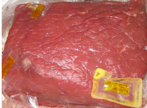
Figure 5- 14 The performance of the final muscle phantom which was used for the MRI scan. A coordinate system was defined for the phantom using three fiducial markers as shown in this picture.
