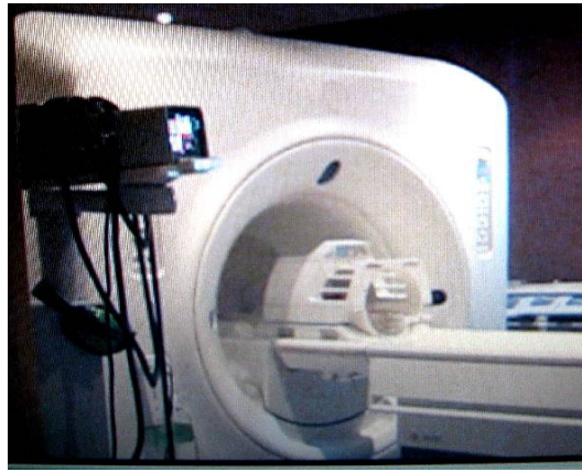
Figure 5- 4 This picture shows the experimental arrangement for the gelatin muscle phantom. The phantom located inside the actuator Type-A was placed inside a head coil. The head coil is shown while it is being inserted inside the MRI bore.
