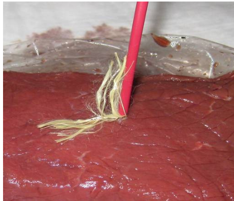
Figure 5- 12 This picture depicts a demonstration of the multi-mode fiber with 1 mm diameter located inside the muscle phantom for twenty minutes in order to heat and create an inclusion using the laser transmission.
