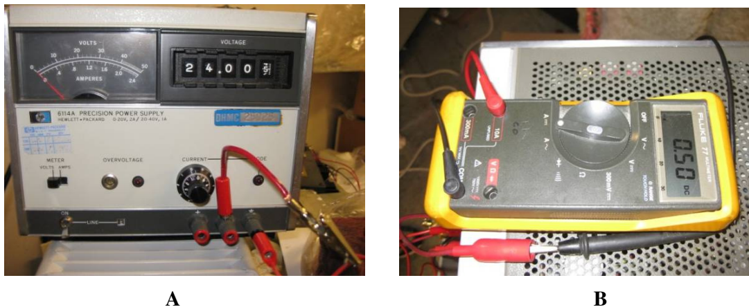
Figure 5- 21 The power supply unit used for this test to provide the voltage (A) and a digital multimeter to measure and adjust the DC current which was passing through the muscle phantom (B), are displayed.
