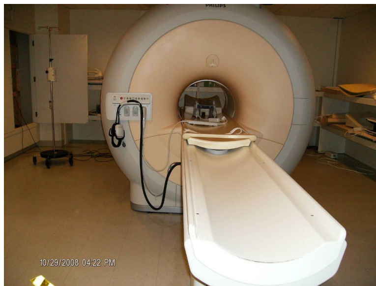
Figure 1- 2 A superconducting magnet from a magnetic resonance imager (MRI)
