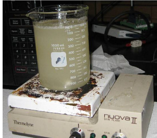
Figure 5- 37 The beaker was placed on the hot plate after removing from the microwave oven to cool down gradually to around 30° C, while a magnetic stirrer was agitating the mixture. This was helpful to remove air bubbles from the gelatin background and obtain a homogenous mixture.
