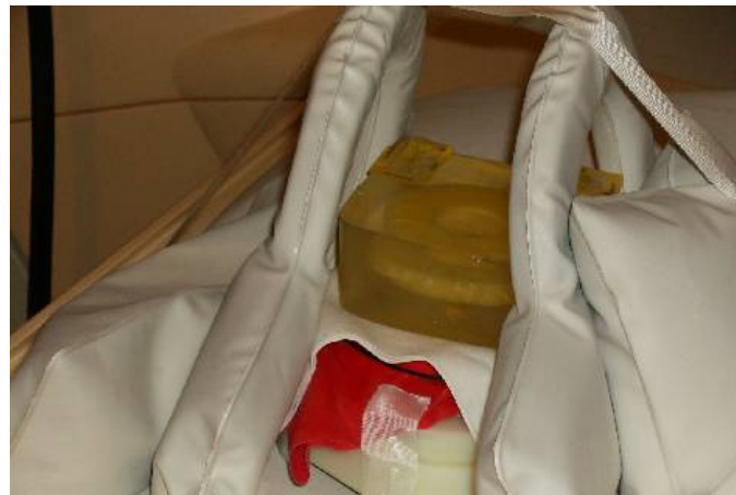
Figure 5- 41 Another view of the same experimental set up for the pineapple gelatin phantom while it has been flipped 90^\circ to capture multiple measurements in 3-D from this orthotropic sample.
