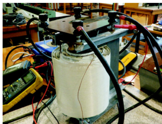
Figure 10. The completed HTS full core transformer
