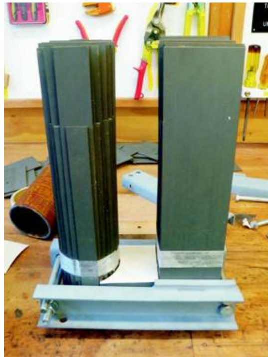
Figure 6. The full core assembly with the top yoke removed.
