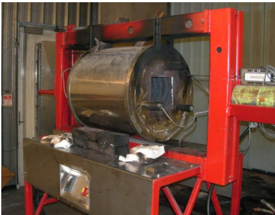
Figure 3-1: Furnace system at the University of Canterbury
