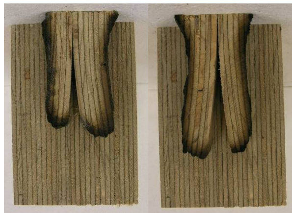
Figure 4-1: Comparative mid-span cross-sectional pictures between the initial and the residual specimens (Left: sample 1; Right: sample 2)
