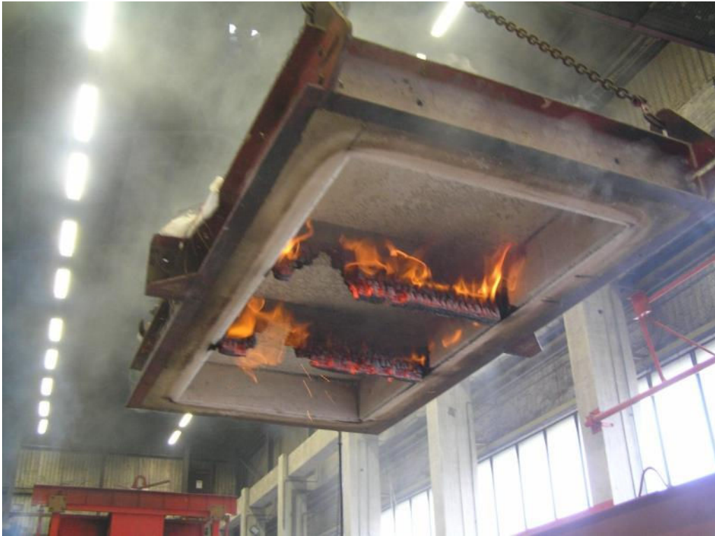
Figure 5-32: Underside of the specimen holder after the fourth pilot furnace test
