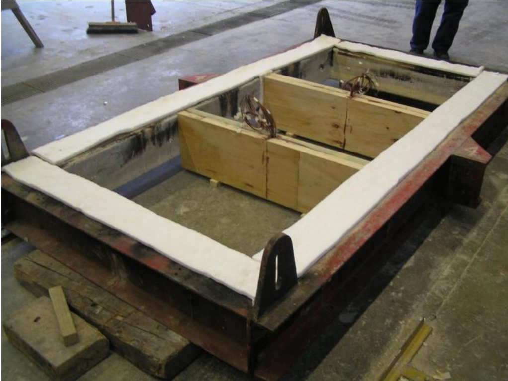
Figure 5-30: LVL specimens installed inside the concrete specimen holder
