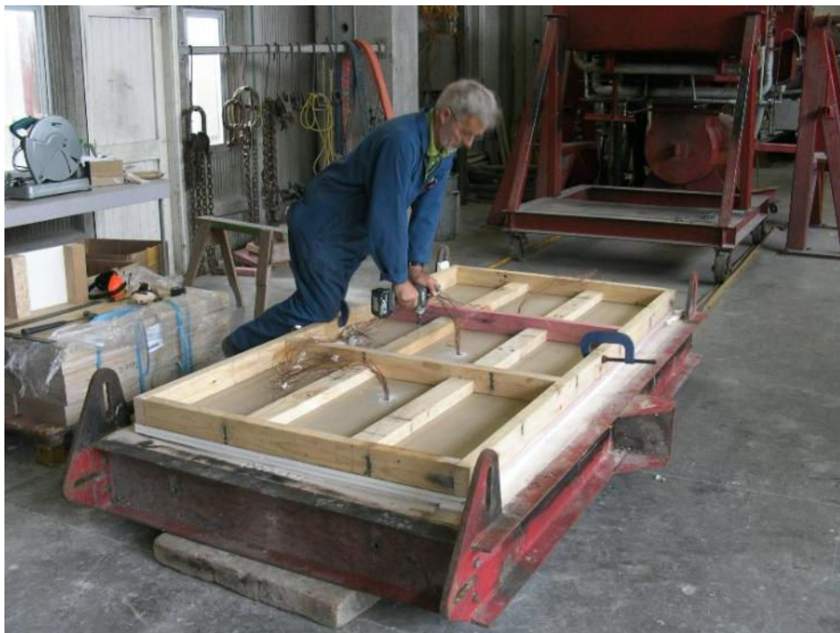
Figure 5-6: Screwing type 17 self-drilling screws through the timber frame into the LVL specimen
