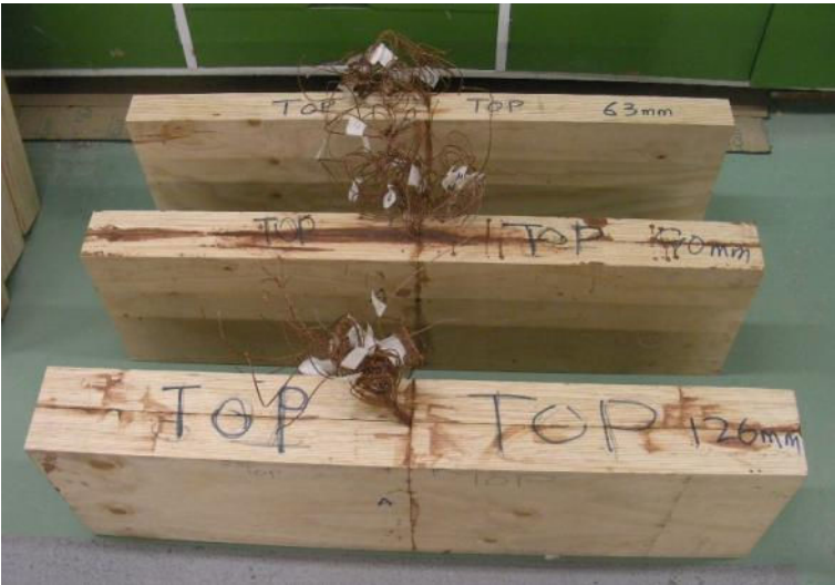
Figure 5-10: Resorcinol adhesive joint after thermocouple instrumentation
