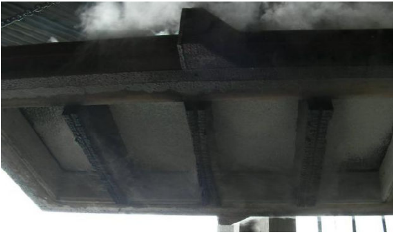
Figure 5-26: Underside of the specimen holder after the third pilot furnace test
