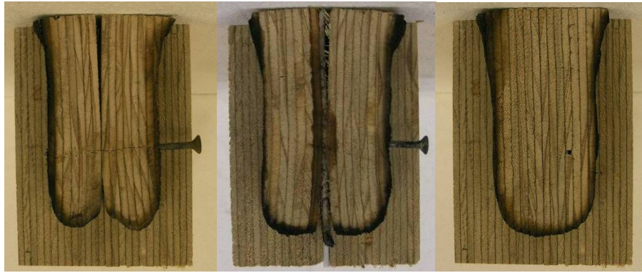
Figure 4-7: Comparative mid-span cross-sectional pictures between the initial and residual LVL specimens (From left to right: screw connected, screw connected with Superwool and glue connected)
