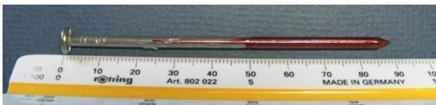
Figure 3-5: Paslode nail used for the small furnace test
