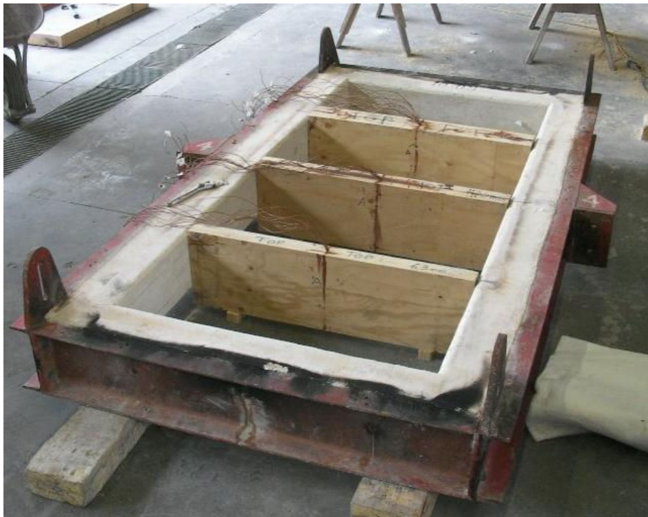
Figure 5-4: LVL specimen installed inside the concrete specimen holder
