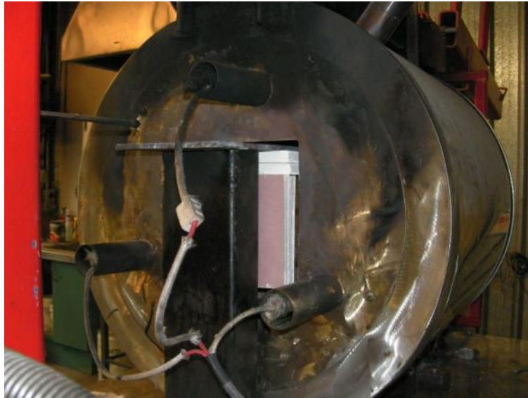
Figure 3-4: Suspending the testing specimen inside the furnace
