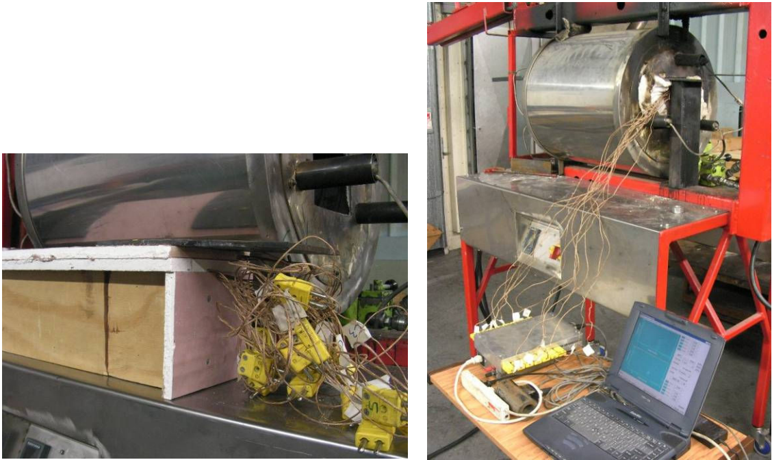
Figure 3-13: Connecting thermocouples to the electronic data recorder
