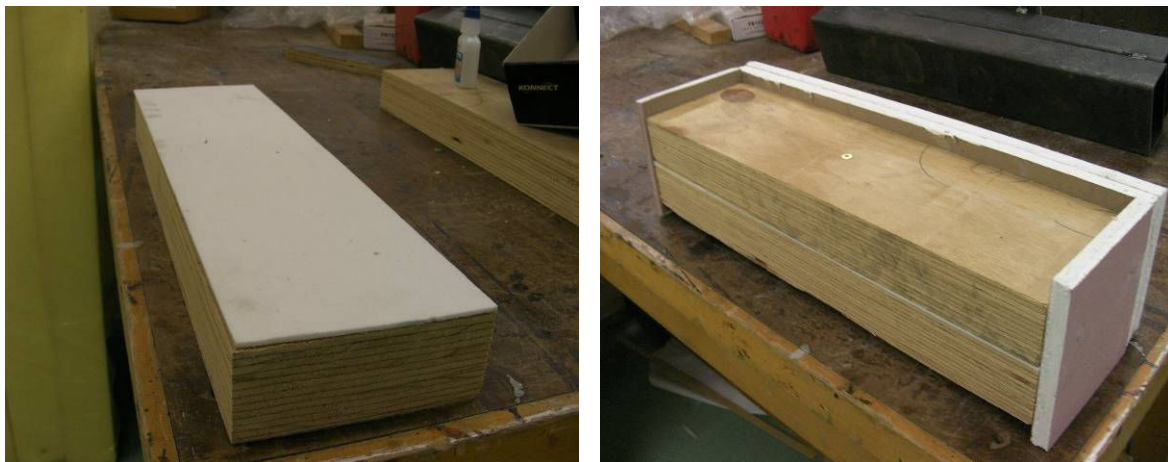
Figure 4-6: (a) Left: Superwool 607 Blanket placed in between the double LVL specimen; (b) Right: Superwool 607 Blanket sandwiched in between the screwed 90mm width double LVL specimen
