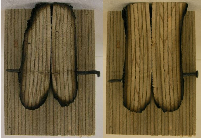
Figure B-2: Nailed Connection (Left: Sample 1; Right: Sample 2)
