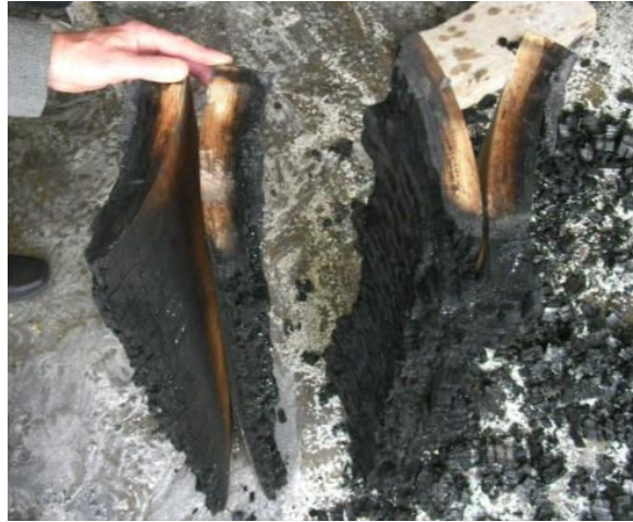
Figure 5-22: Separation of Samples 2 (left) and 3 (right) after the second pilot furnace test
