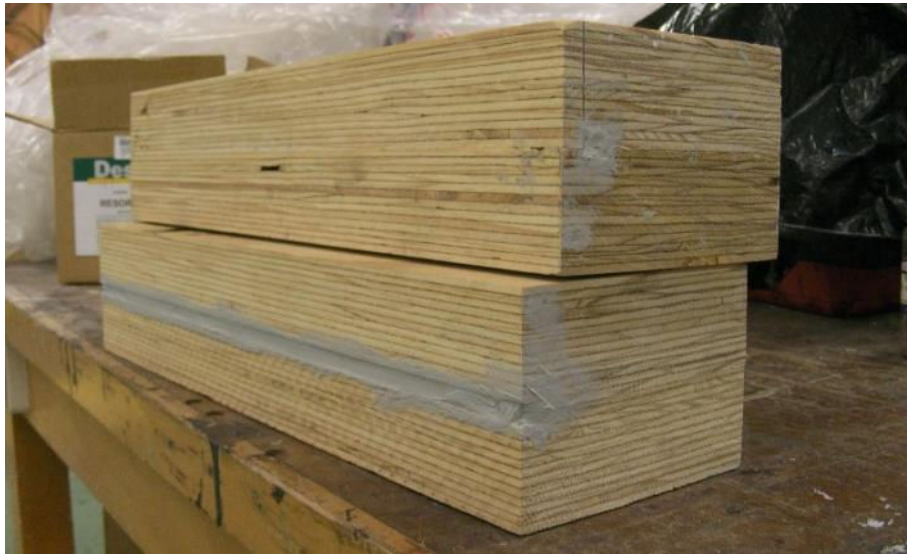
Figure 4-9: A picture showing the constructed LVL specimens for the two intumescent sealant channels (Top: Layout 2; Bottom: Layout 1)
