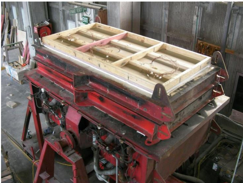
Figure 5-8: The complete assembly placed above the pilot furnace ready for testing
