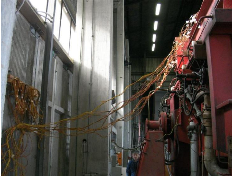
Figure 5-12: Connecting thermocouples to the electronic data recorder
