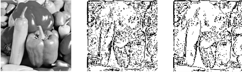
FIGURE 2-9: An image (left), its edge map (middle) and its edge map with variance thresholding applied (right). Notice some intra-texture edges have been suppressed. Reproduced from Ahmed and Choi (1999).
