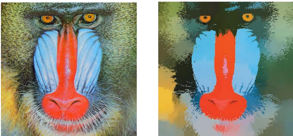
FIGURE 3-12: The mean-shift filter (right) run on the mandrill image (left). Images from Comaniciu and Meer (2002).
