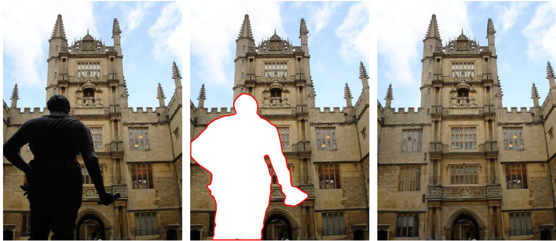
FIGURE 1-7: Boundary detection can be used to identify where inpainting should occur. Reproduced from Whyte et al. (2009)
