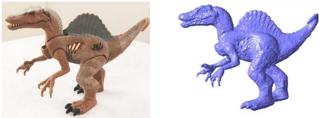
FIGURE 1-4: The object shown in the left image was sculpted into a visual hull (right) using boundary detection. Reproduced from Furukawa and Ponce (2009).
