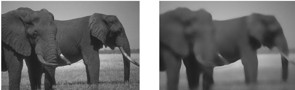
FIGURE 3-7: The Nitzberg operator (right), applied to an image (left). These images are greyscale, but it is possible to use the Nitzberg operator on colour images as well.
