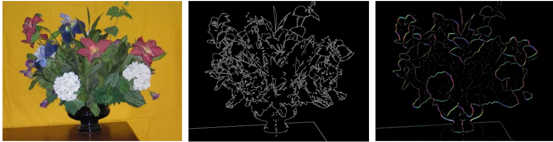
FIGURE 2-1: An image (left), its edge map (middle) and its boundary map (right). The edge map was generated using the Canny edge detector (section 2.4), and the boundary map was generated using the Variance Ridge Detector (proposed in chapter 6).
