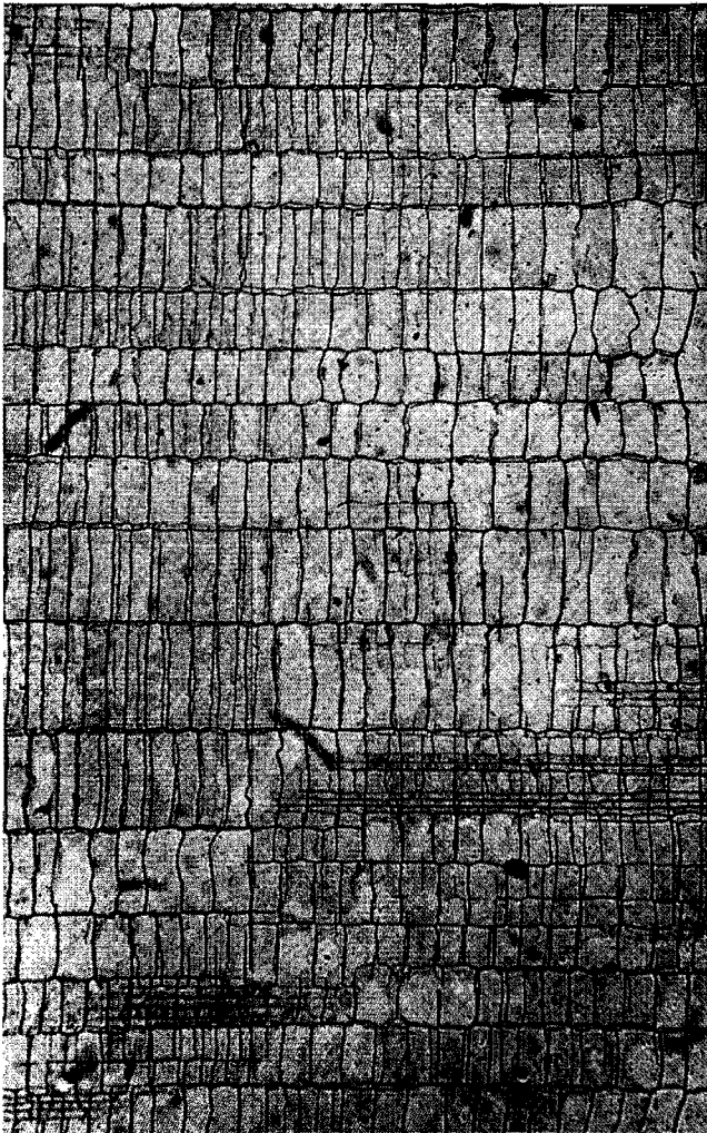
FIG. 4—Radial longitudinal section of the secondary xylem through parenchyma. ( \times 44 )
