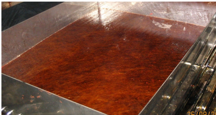
Figure 25: GRP, dark brown colour at the end of the 300°C test
