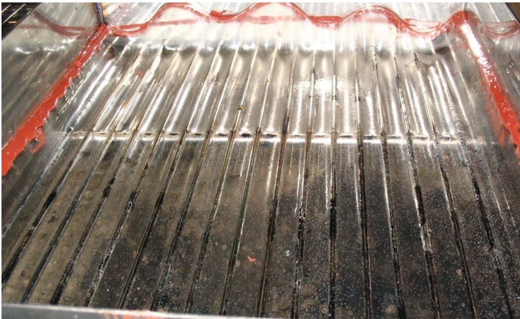
Figure 20: The slumped polycarbonate after 15 minutes exposure at 250°C
