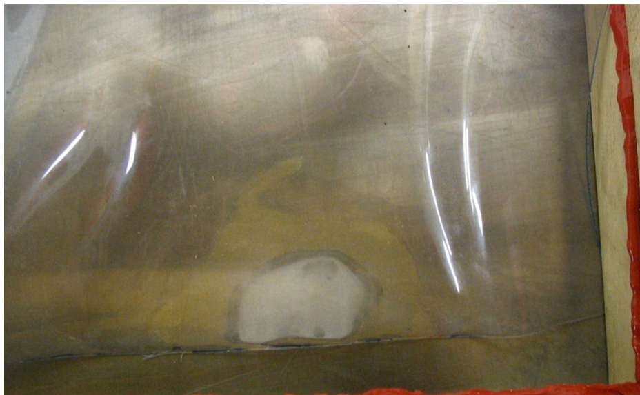
Figure 15: PVC after 50 minutes exposure at 150°C
