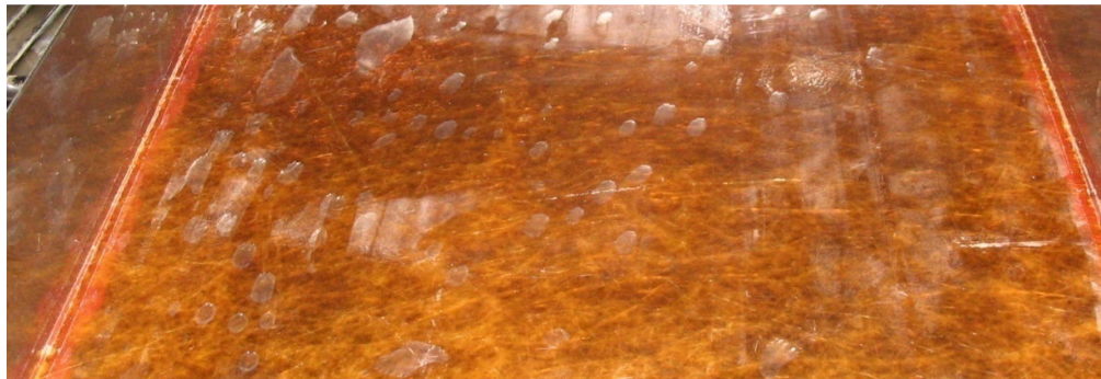
Figure 24: GRP, bubbles formed during the test at 250°C
