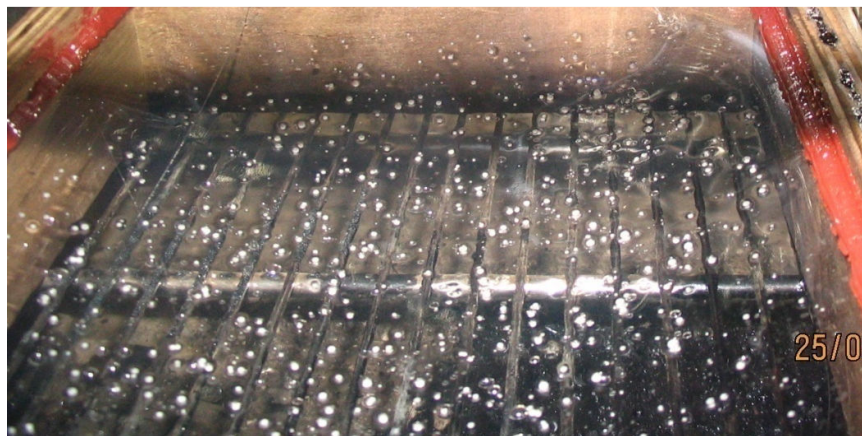
Figure 23: Deterioration of the acrylic at 250°C
