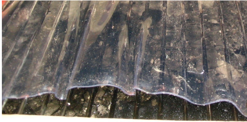
Figure 16: The PVC shrinking from the first side after 10 minutes exposure to 200°C
