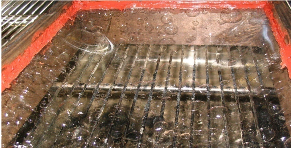
Figure 22: The large bubbles formed during the acrylic test at 200°C
