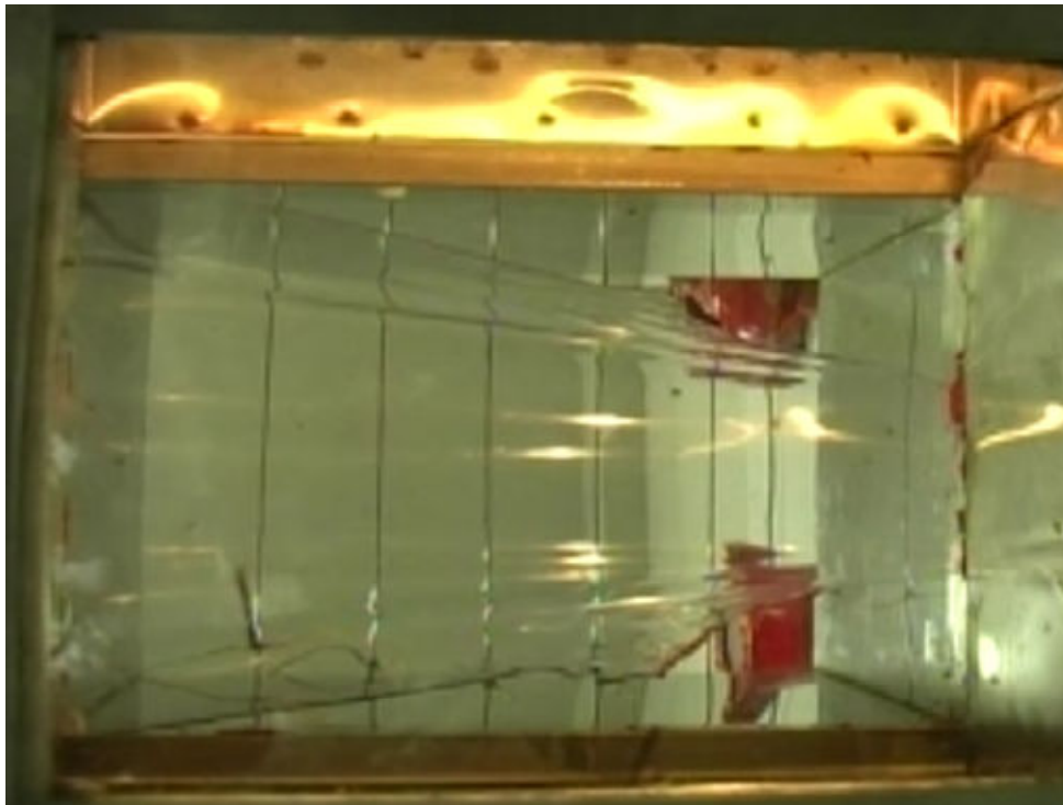
Figure 40: Image of deformed sample, test 1, and note flow is from bottom to top
