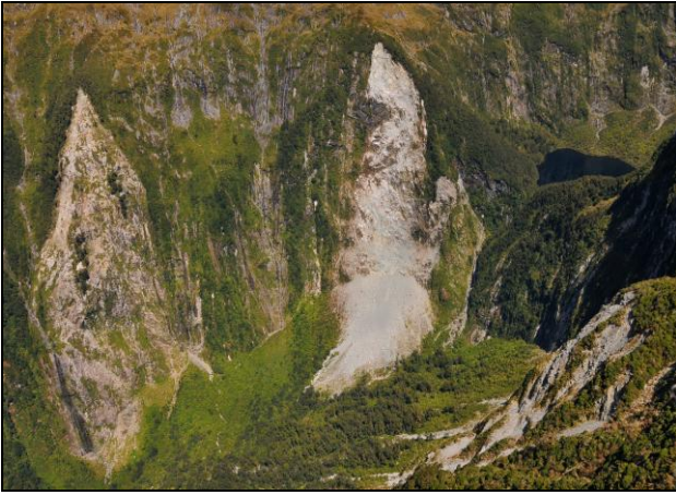
Figure 24: The head of this large 2003 landslide (centre) at the head of First Arm was reactivated by the 2009 earthquake, but the 2003 landslide to the left and others nearby were not obviously affected. Less than ~20% of the 2003 slides appear to have been significantly reactivated by the 2009 earthquake. This is currently being investigated using satellite imagery.
