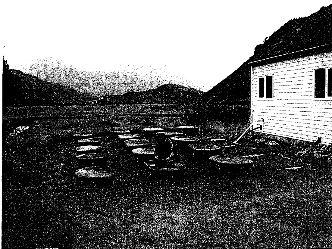
Figure 4.8. Experimental set-up of the sixteen tanks at the Cass field station. Water was pumped from Grasmere Stream (left) into the tanks. Fifteen tanks were used for the experiment.
