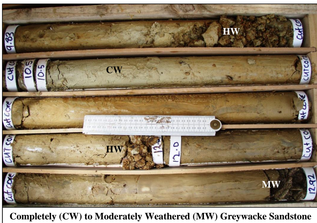
Figure 4.2: Retrieved core from Borehole 1 (S Semmens 2008).
