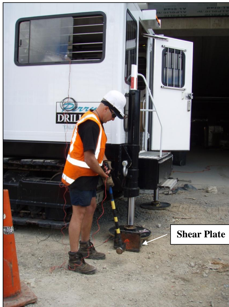
Figure 4.5: Shear wave generation (S Semmens 2009).
