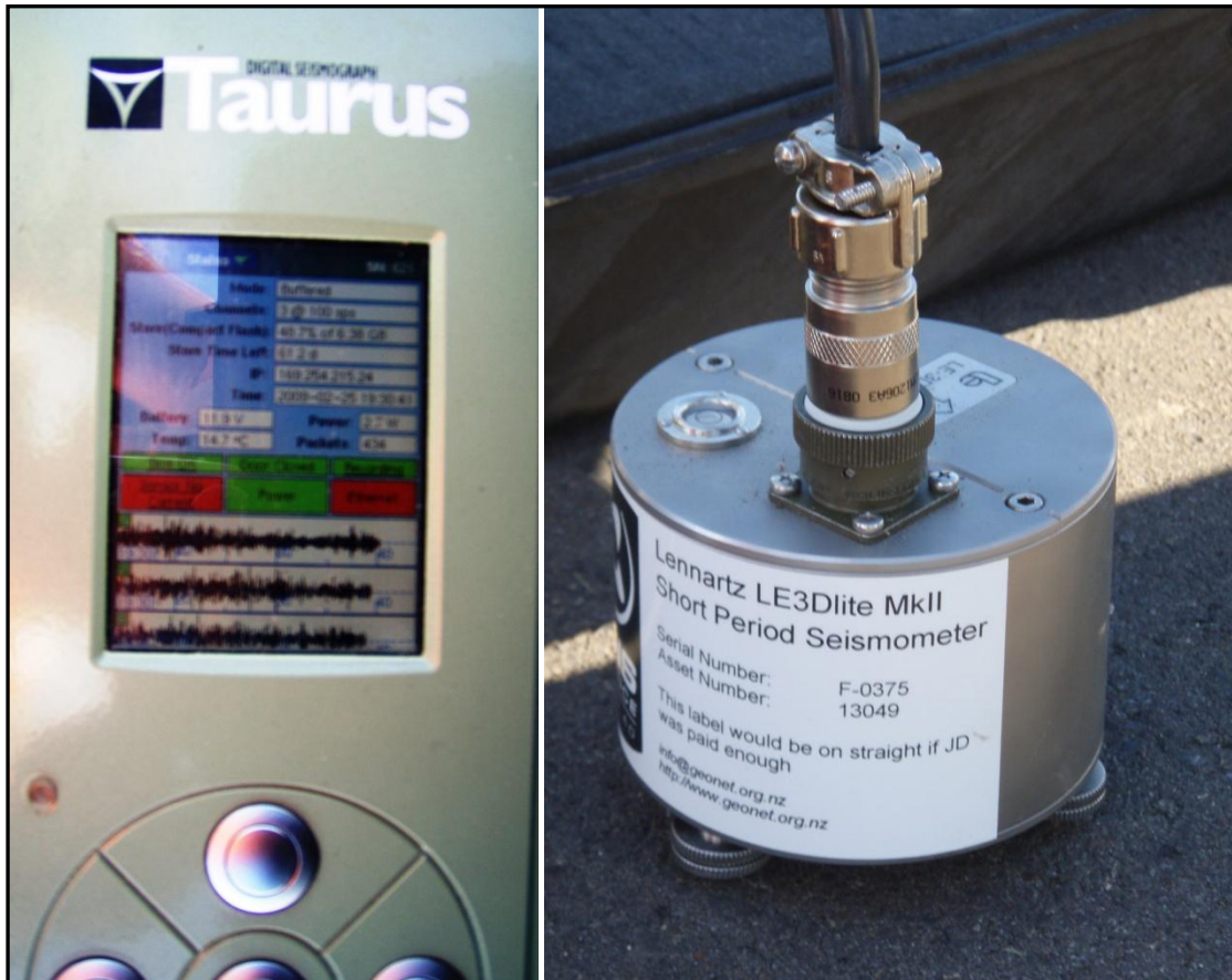
Figure 4.9: Lennartz Seismometer and Taurus portable digital seismograph recording (S Semmens 2009).
