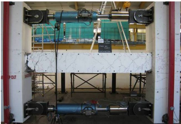
(a) Damage between Column A and Column B
