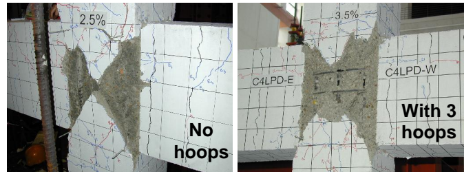
Figure 5. Specimens at the end of the tests
