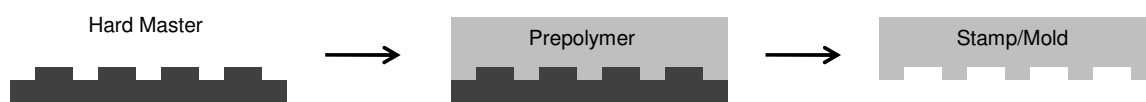
Scheme 6.1. General procedure for fabricating stamps and molds for use in soft lithography.
