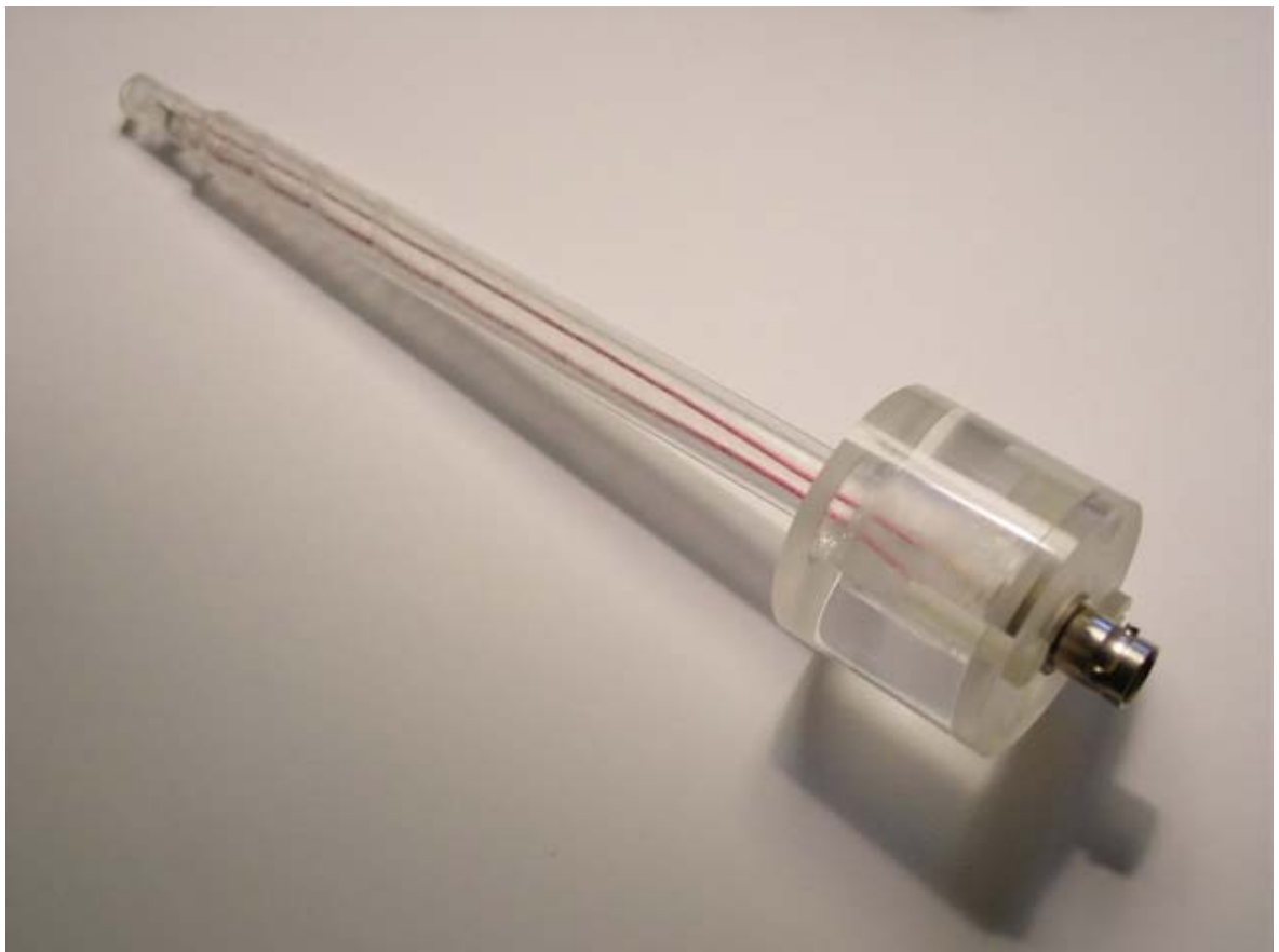
Figure 3.10. Thin Perspex detector using free air wire attachment.
