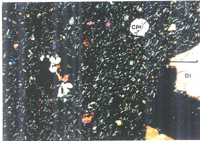
Fig. 3.13 Strongly embayed olivine phenocryst (ol) adjacent to clinopyroxene phenocryst (cpx) in olivine-basalt M36B4036, (c.p.l) scale = 1 mm.
