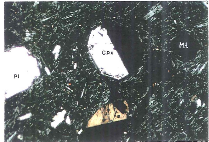
Fig. 3.10 Euhedral clinopyroxene (augite) in late phase Lyttelton hawaiite M36B4018, (c.p.l) scale = 1 mm.
