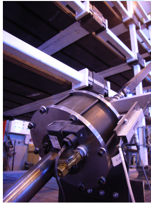
Figure 7: Closeup of a resettable device installed on the test structure. The linear transducer on the left side measures displacement across the device from which relative ( 3^{rd} ) floor motion (to ground) can be inferred.
