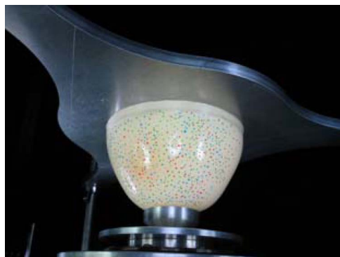
Fig. 18. Silicon phantom under actuation with colored dots applied.
