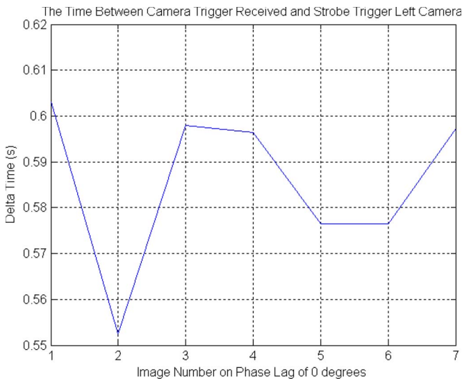
Fig. 7. Graph of the dSpace trigger pulse/strobe trigger pulse time period.
