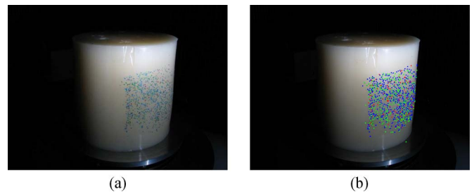
Fig. 16. (a) Silicone gel phantom with colored speckles. (b) Detected RGB points.
