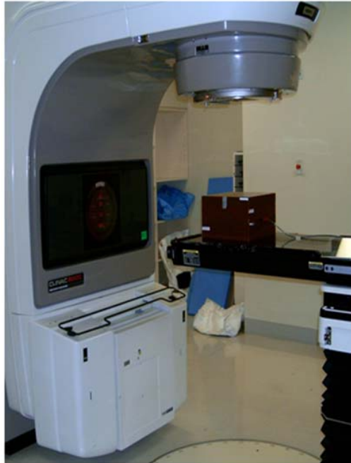
Figure 3.3 Experimental setup of the CVD diamond detector in the water phantom for a 6 MV photon beam
