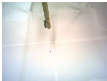
Figure 4.4: A pole with a laser mounted at the bottom. The laser dot projected on the ground has been enhanced in the photo to make it more visible.
