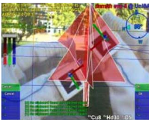
(c) Object manipulation with the Tinmith glove [Piekarski 2004]
