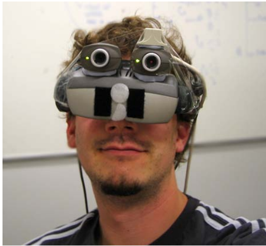
(a) The stereo video see-through HMD
