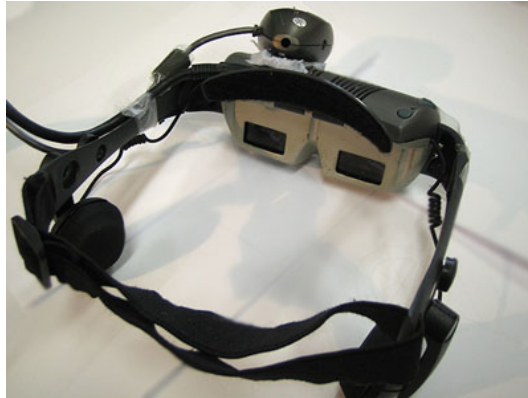
Figure 2.2: The i-glasses, a video HMD, with a webcam attached at the top.
