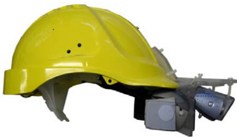
(a) The helmet from the side, showing that the camera was angled at the ground
