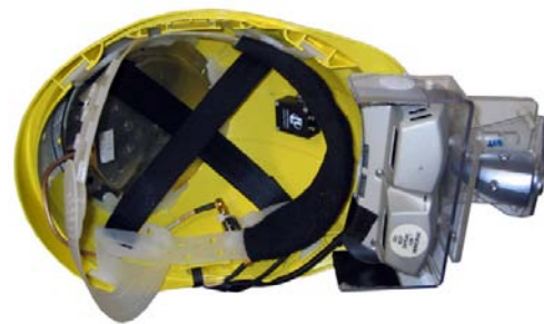
(b) The inside of the helmet showing the round GPS antenna, the small InertiaCube, the i-glasses and the camera.
