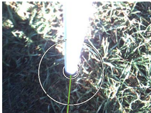
(c) A bull's eye helped the user to place the pole accurately on the point. A green line highlighted the path to the next target.
