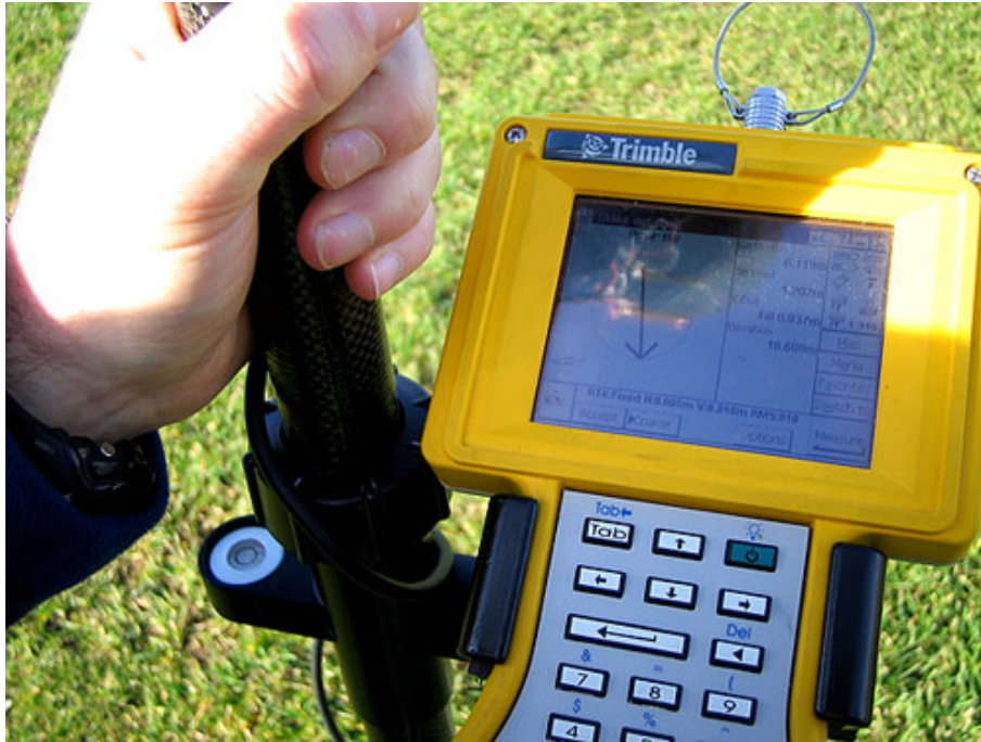
Figure 2.19: The TSC attached to a surveying pole seen from the user's perspective. The water level is the white circle to the left of the pole.
