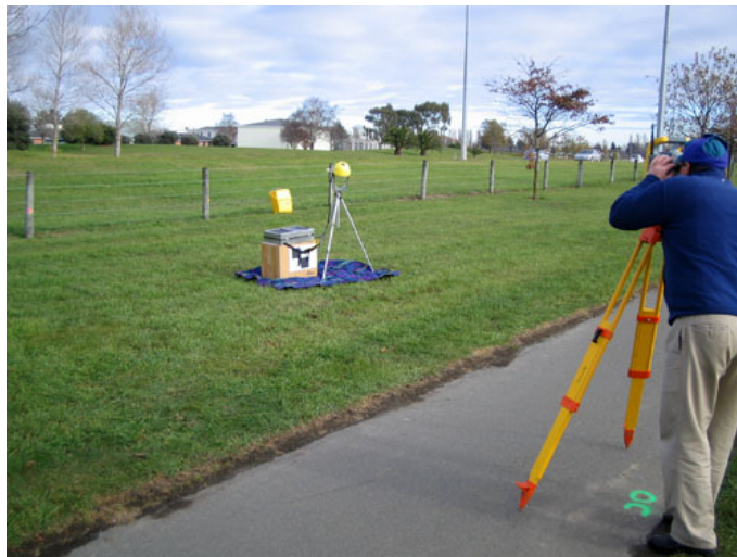
(b) Surveying the calibration points with an optical total station.
