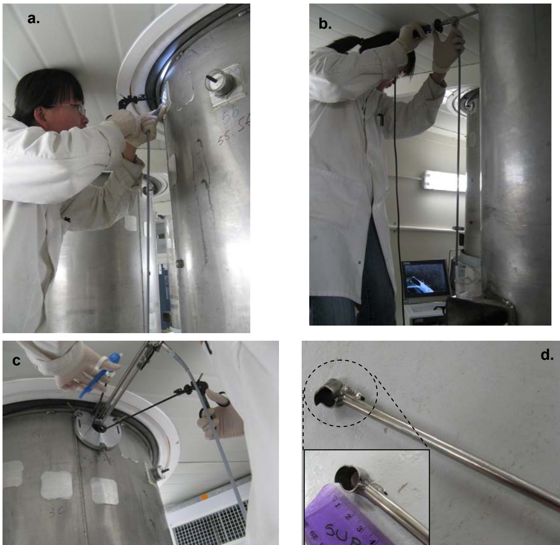
Figure 4.3 a). Placing the AEM-Whatman 3MM strip on top of roots for OA collection using long armed forceps under the endoscope light source. b). Checking the AEM-Whatman 3MM strip after being placed on top of roots for OA collection using the endoscope camera system. c). Removing AEM-Whatman 3MM from the root/soil samples and sampling root samples with long arm scissors. d). A specially designed soil sampler for non-rhizosphere soil sampling in access portals.
