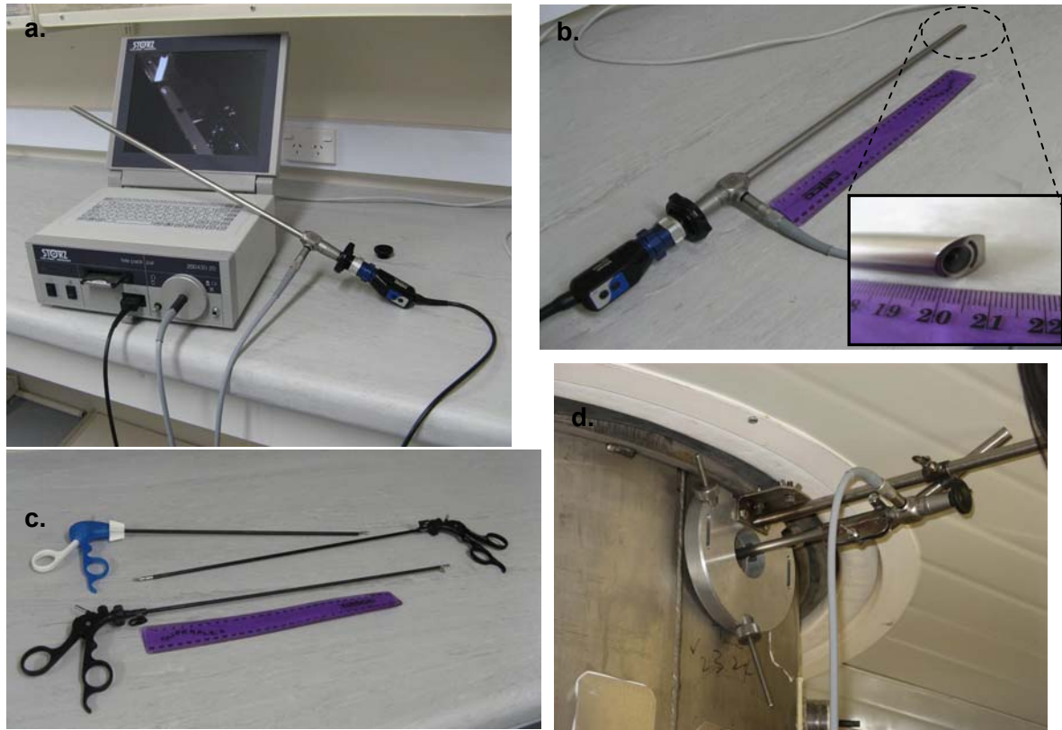
Figure 4.2 a). The endoscope system. b). The camera lens (45 cm long, 1 cm diameter). c). Long armed scissors and forceps (approximate 45 cm long) used during the second sampling. d). Specially designed endoscope lens-rhizotron adapter that can hold the lens in the access portal and allow the lens be able to rotate 360° and move along the access portal.
