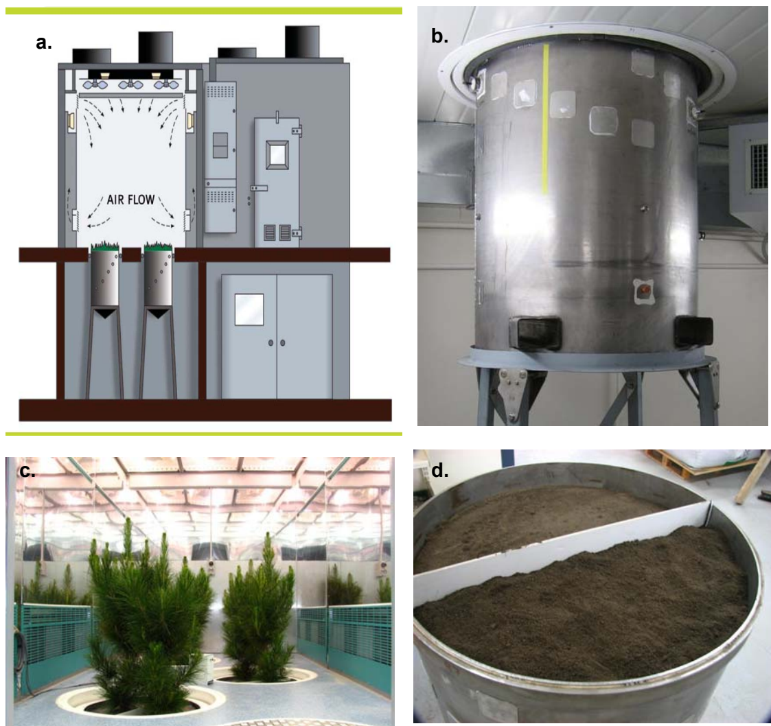
Figure 3.1 a). Rhizotron system in the New Zealand Biotron facility. Left: cross section view of a growth room positioned above a rhizotron room. Right: front view of a growth room positioned above a rhizotron room. b). Stainless steel rhizotron cylinder in the downstairs rhizotron room. c). Pinus radiata in the upstairs growth room after one year growth. d). Packing the soil into the rhizotron which has been divided into two halves.
