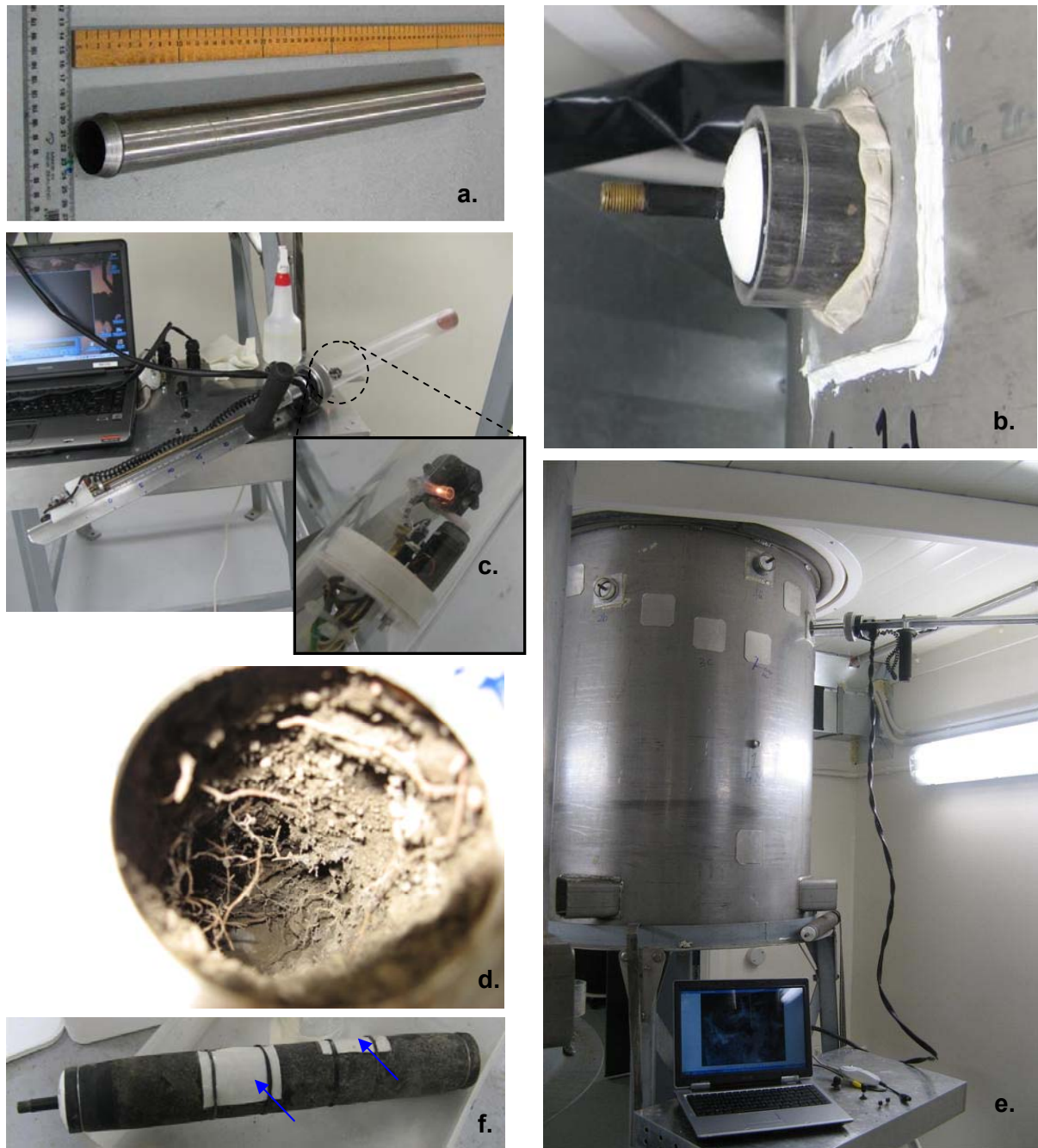
Figure 3.2 a). The soil corer used for creating access portals in the rhizotron. b). The physical integrity of the access portal is maintained using a removable inflatable tube between samplings. c). The sealed motorised camera system for image and position recording, with a close up of a motorised camera inside the perspex tube. d). The access portal after removing the inflatable tube for root monitoring or sampling. e). The camera system recording the root image in the access portal. f). AEM strips backed with Whatman 3MM (indicated by blue arrows) fixed on an inflatable tube for root exudates collection in the access portal.
