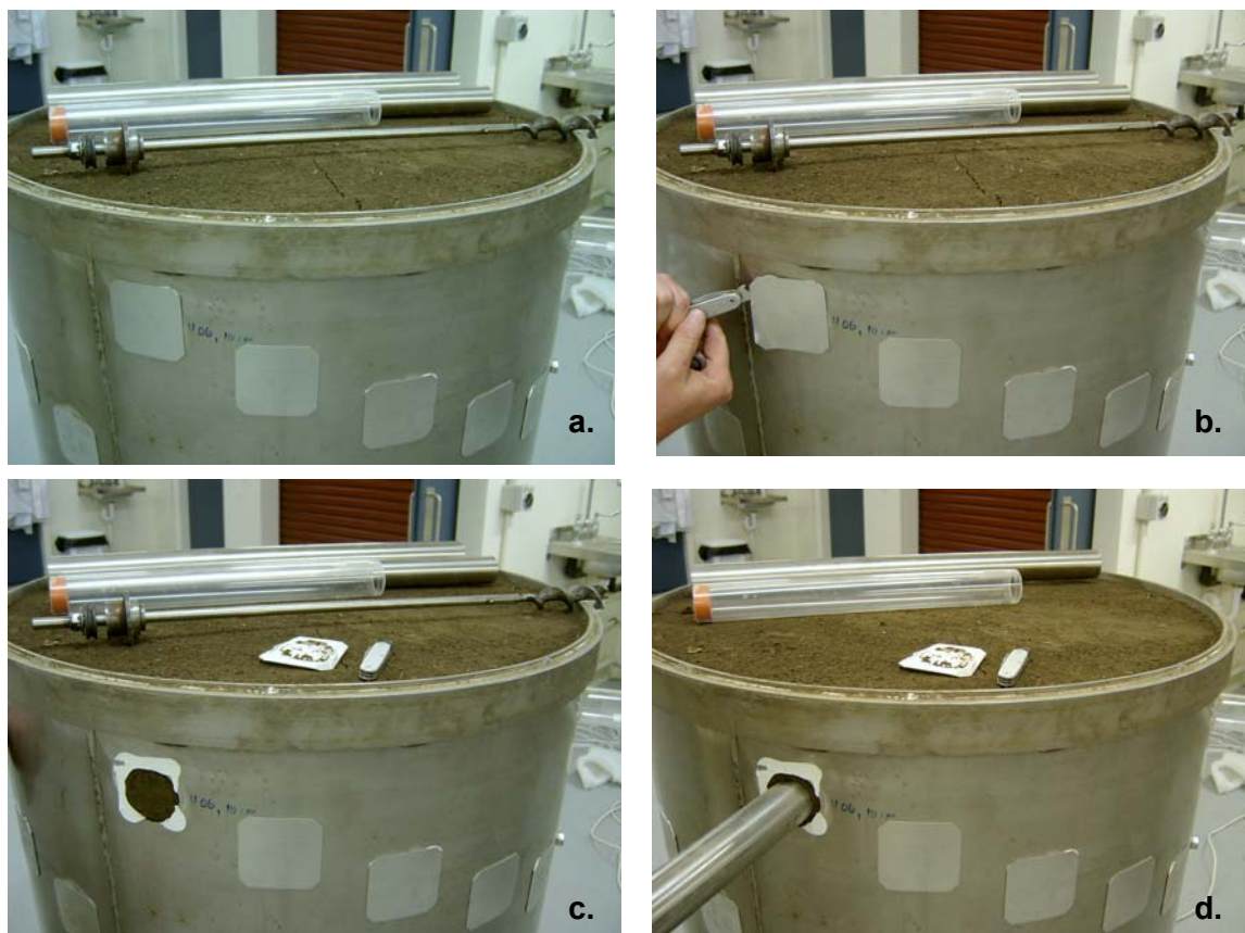
Figure A3.5-1 Creation of the horizontal access portal in a rhizotron. a). The rhizotron packed with soil. b). Removing the plate on the rhizotron wall. c). Shown is the pre-existing opening in the rhizotron with soil after removal of the plate. d). A soil corer is inserted into the rhizotron through the original opening to create an access portal.
